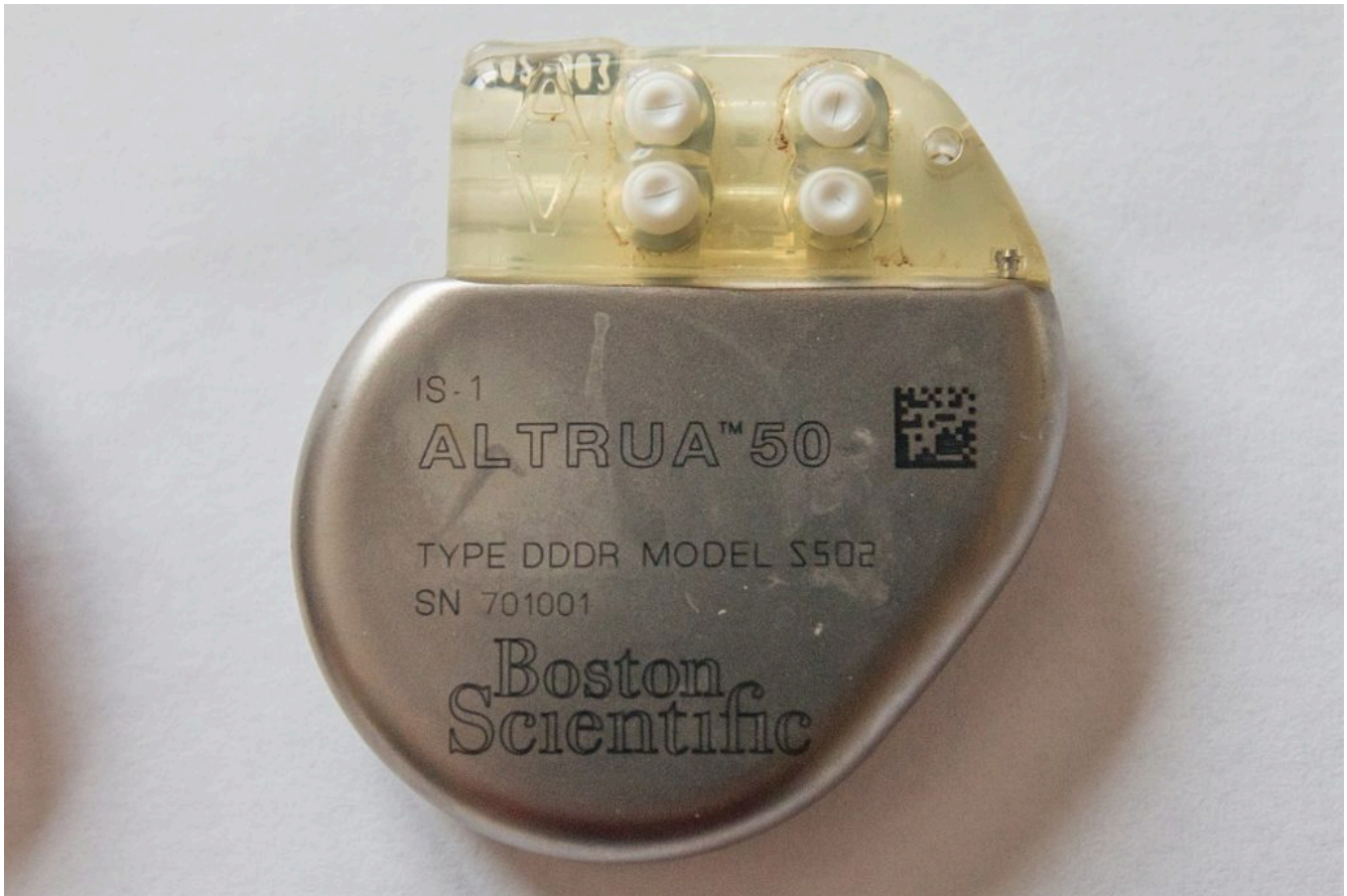
Figure 16.6: Technology encompasses more than just information technology. This pacemaker utilizes information technology to record heart-function data a doctor can read later. But the product might also utilize other new technologies, such as a new battery, materials used to connect the pacemaker to the heart, and the casing for the pacemaker, all of which affect its performance. “ Boston Scientific Altrua 50 Dual-chamber cardiac pacemaker ” by Johannes Maximilian , CC-BY-NC-ND
