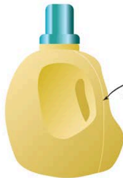
PARTING LINES ON INJECTION MOLDED PLASTICS
