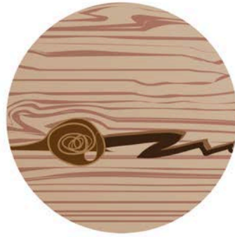
LOOSE KNOTS AND CRACKS IN WOOD
