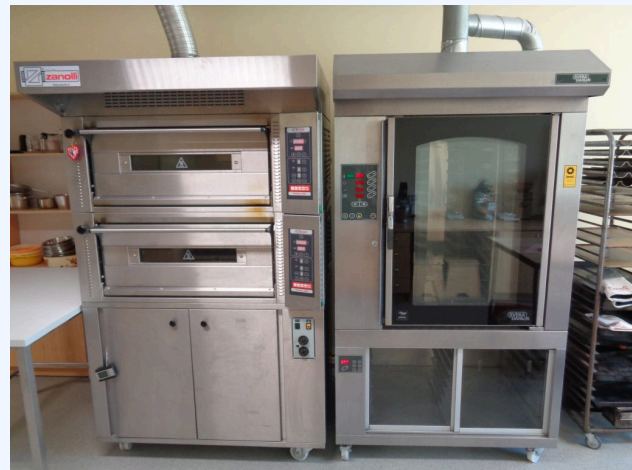
Figure 3.1.2 "Industrial hearth deck oven and rotary rack oven" by Turaidis, CC BY-SA 4.0
