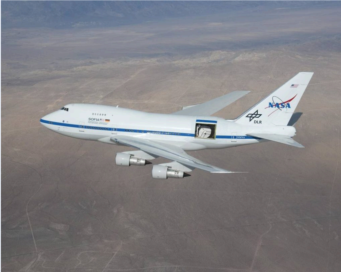
Figure 4.26. SOFIA allows observations to be made above most of Earth's atmospheric water vapour. SOFIA by NASA, NASA Media Licence.
