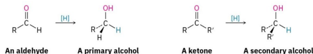
Figure 23.3i. An aldehyde is reduced to a primary alcohol. A ketone is reduced to a secondary alcohol ( Organic Chemistry , CC BY-NC-SA 4.0 )
