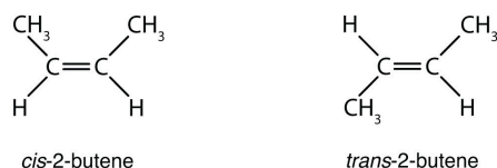
Figure 22.2d. Models of (left) Cis -2-Butene and (right) Trans -2-Butene. (Credit: Intro Chem: GOB (V. 1.0) , CC BY-NC-SA 3.0).
