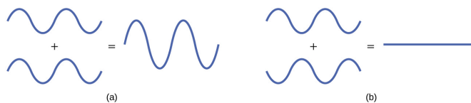
Figure 21.4c. (a) When in-phase waves combine, constructive interference produces a wave with greater amplitude. (b) When out-of-phase waves combine, destructive interference produces a wave with less (or no) amplitude (credit: Chemistry (OpenStax), CC BY 4.0 ).
