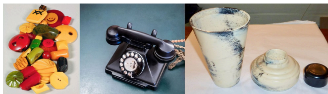
Figure 27.1f. Examples of products made from Bakelite (credit a: “ Set of Phenol formaldehyde resin buttons ” by Gregory Tobias, CC BY-SA 3.0 ; b: work by William Warby, CC BY 2.0 ; c: work by Tangerineduel, CC BY-SA 4.0 ).
