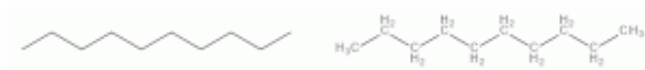
Figure B2: Line structure and condensed structural diagram for decane ( C_{10}H_{22} ). Drawn with BIOVIA Draw.
