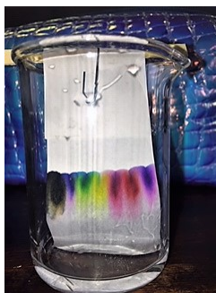
Figure 29.1a. Picture of paper chromatography of various marker ink. (Credit: Photo by Amitchell125, CC BY-SA 4.0 )
