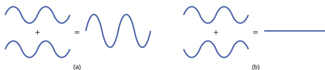
Figure 21.4c. (a) When in-phase waves combine, constructive interference produces a wave with greater amplitude. (b) When out-of-phase waves combine, destructive interference produces a wave with less (or no) amplitude (credit: Chemistry (OpenStax) ( https://openstax.org/books/chemistry/pages/8-4-molecular-orbital-theory ), CC BY 4.0).
