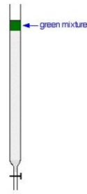
Figure 29.3b. Start of a chromatography column with a green mixture (credit: Chromatography , CC BY-NC 4.0).
