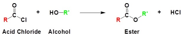
Figure 25.3s. Formation of an ester from substitution of an acid chloride with an alcohol (credit: UIS: CHE 269 (Morsch and Andrews) , CC BY-NC-SA 4.0).
