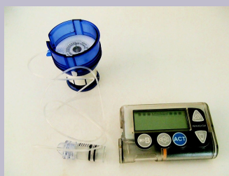
Figure 28.3a. Insulin pump, showing an infusion set loaded into spring-loaded insertion device. A reservoir is attached to the infusion set (shown here removed from the pump). (Photo by David-i98, PDM).
