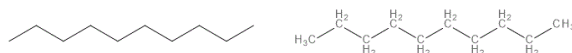
Figure B2: Line structure and condensed structural diagram for decane ( C_{10}H_{22} ). Drawn with BIOVIA Draw.
