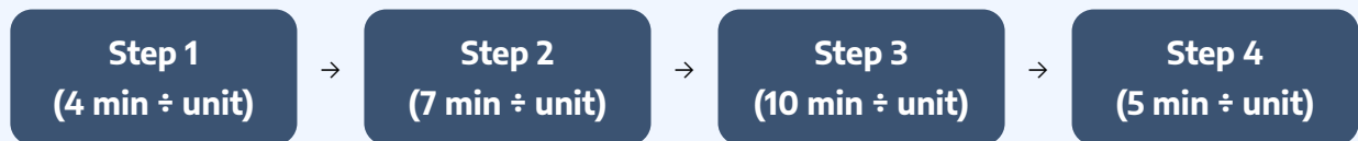
Figure 4.9.1 Flow diagram depicting the time taken for each step of Caroline's manufacturing process.
