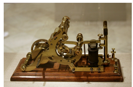
Antique automatic telegraph receiver made of metal and wood. Source: Automatic Telegraph Receiver by Cliff, CC BY 2.0
