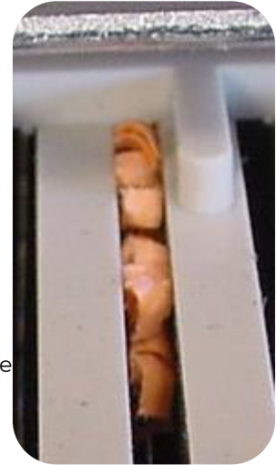
“A chad jam in a Votomatic punch, seen from behind” by Douglas W. Jones . Used under FDEd(Can) .
