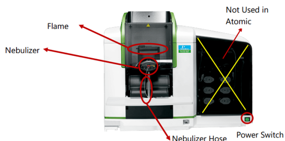
Figure 6.1.3. Main Components of PinAAcle 900F Perkin Elmer Flame Emission Spectrometer. Image by T. Sarchami, CC BY-NC-ND 4.0. Click to enlarge .
