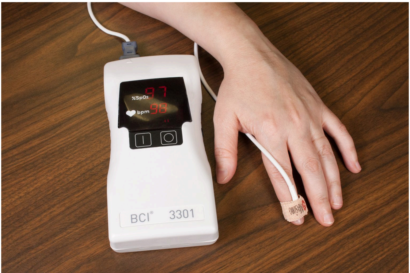
Figure 6.5.2: Pulse oximeter with sensor taped around finger
