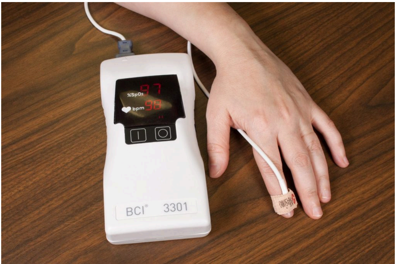
Figure 6.5.2: Pulse oximeter with sensor taped around finger
