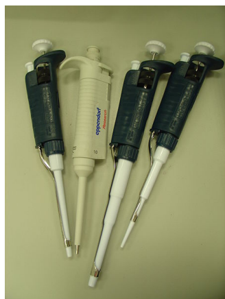
Figure 2.6 Digital micropipets. From the left, the pipets deliver volumes of 500 \mu\text{L} –200 \mu\text{L} ; 0.5 \mu\text{L} –10 \mu\text{L} ; 1000 \mu\text{L} –100 \mu\text{L} ; 1 \mu\text{L} –20 \mu\text{L} . Source: Retama (commons.wikimedia.org).
