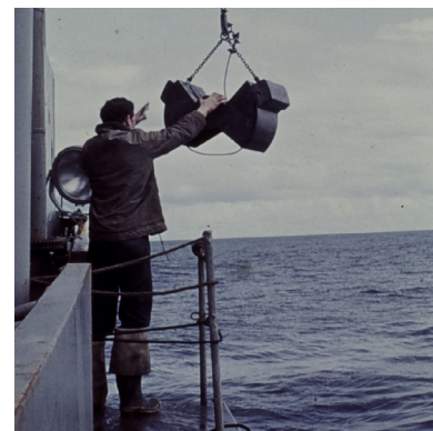
Figure 7.7 Bottom grab sampler being prepared for deployment. Source: NOAA (photolib.noaa.gov).
