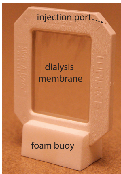
Figure 7.14 Example of a dialysis cassette. The dialysis membrane in this unit has a molecular weight cut-off of 10 000 g/mol. Two sheets of the membrane are separated by a gasket and held in place by the plastic frame. Four ports, one of which is labeled, provide a means for injecting the sample between the dialysis membranes. The cassette is inverted and submerged in a beaker containing the external solution, which is stirred using a stir bar. A foam buoy, used as a stand in the photo, serves as a float so that the unit remains suspended above the stir bar. The external solution is usually replaced several times during dialysis. When dialysis is complete, the solution remaining in the cassette is removed through an injection port.
