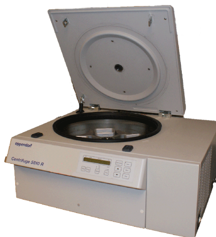
Figure 7.15 Bench-top centrifuge capable of reaching speeds up to 14 000 rpm and centrifugal forces of 20\,800 \times g . This particular centrifuge is refrigerated, allowing samples to be cooled to temperatures as low as -4^{\circ}\text{C} .
