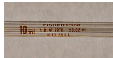
Figure 2.8 Close-up of the 10-mL transfer pipet from Figure 2.5.
