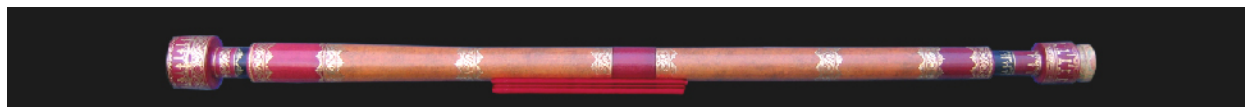
Figure 2.20. Telescope Used by Galileo. The telescope has a wooden tube covered with paper and a lens 26 millimeters across.
