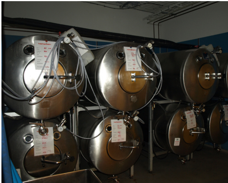
Figure 4.22 Fermentation of grape juice to make wine produces CO 2 as a byproduct. Fermentation tanks have valves so that pressure inside the tanks can be released.
