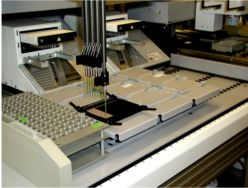
Figure 10.17 This machine is preparing to do a proteomic pattern analysis to identify specific cancers so that an accurate cancer prognosis can be made. (credit: Dorie Hightower, NCI, NIH)
