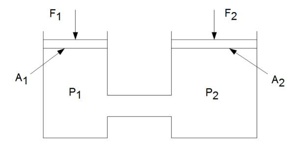
Figure 4.7: A simple hydraulic system.
