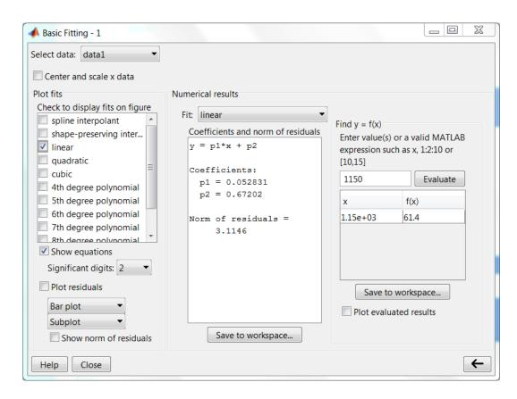
Figure 7.6: Estimating the Voltage that corresponds to a Temperature of 1150 C.
