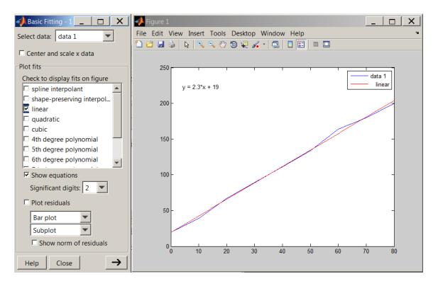
Figure 7.4: Basic Fitting window is used to select the desired regression analysis parameters.
