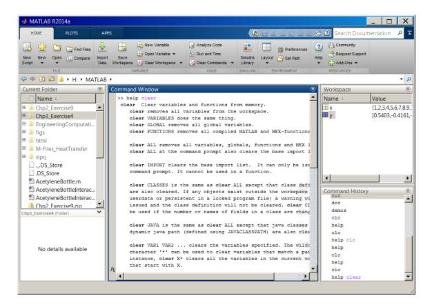
Figure 1.15: The output of  $\gg$  help clear command.
