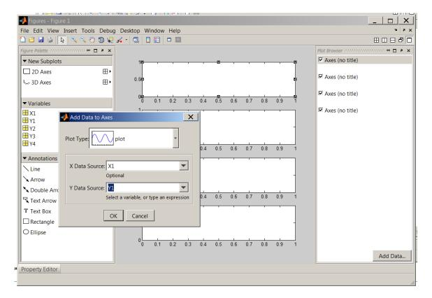
Figure 3.7: Adding data to axes.
