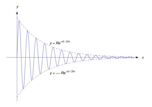
Figure 6.2.1 Underdamped motion
