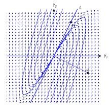
Figure 10.5.4 Negative eigenvalue; motion toward Figure 10.5.5 Negative eigenvalue; motion toward the origin the origin
