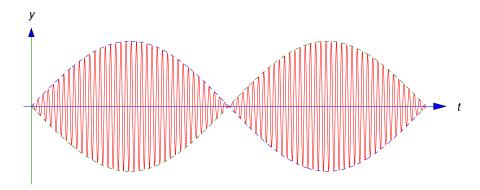
Figure 6.1.6 Undamped oscillation with beats
