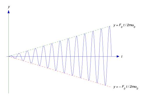
Figure 6.1.7 Unbounded displacement due to resonance
