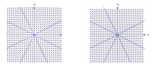
Figure 10.4.1 Trajectories of a  $2 \times 2$  system with a Figure 10.4.2 Trajectories of a  $2 \times 2$  system with a repeated positive eigenvalue repeated negative eigenvalue
