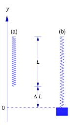
Figure 6.1.3 (a) Natural length of spring (b) Spring stretched by mass
