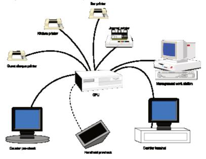
Figure 38: POS terminals connected to central processing unit
