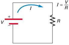
Figure 7.1. Schematic for a simple circuit.
