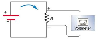
V = IR = 18 V Figure 7.2. The voltage drop across a resistor in a simple circuit equals the voltage output of the battery.
