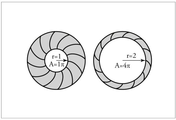
**Figure 14-7**. The camera's aperture controls the amount of light admitted to the sensor and also affects the depth of field, the depth of scene that's in focus from front to back. Smaller apertures (left) admit less light but provide greater depth of field.
