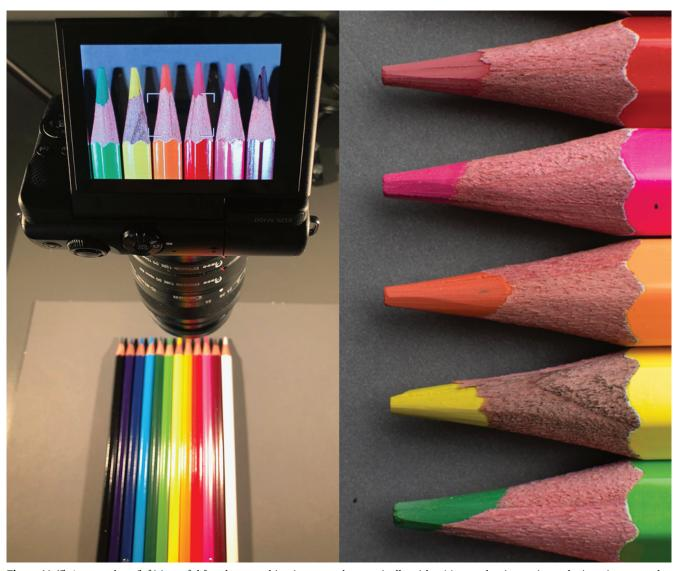
Figure 14-15. A macro lens (left) is useful for photographing items up close, typically with a 1:1 reproduction ratio, so the item is captured in its actual size (right) on the sensor. Photos Richard Adams. Image licensed under CC BY 4.0.
