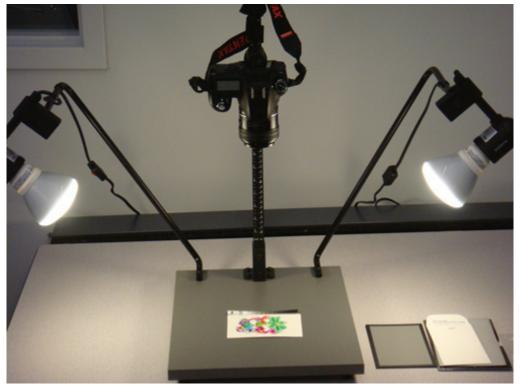
**Figure 14-10**. A copy stand is useful for photographing flat objects. Two lights at 45° angles help reduce glare from the subject's surface. Photo Richard Adams. Image licensed under CC BY 4.0.
