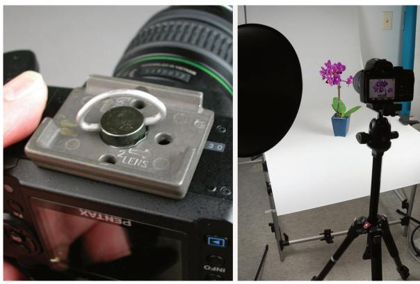
Figure 14-5. Quick-release tripod mount includes a plate that screws into the camera mount and then clips onto the tripod, allowing for rapid on-and-off operation. Photos Richard Adams. Image licensed under CC BY 4.0.
