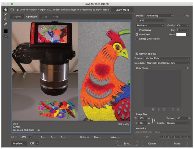
Figure 15-4. Photoshop's Export > Save for Web dialog box offers the opportunity to customize the image format (upper right corner) and size (lower right) and also includes a prediction of download time (lower left) at various internet bandwidths. Photo Richard Adams. Image licensed under CC BY 4.0. Adobe® Photoshop® screenshot(s) reprinted with permission from Adobe Systems Incorporated.
