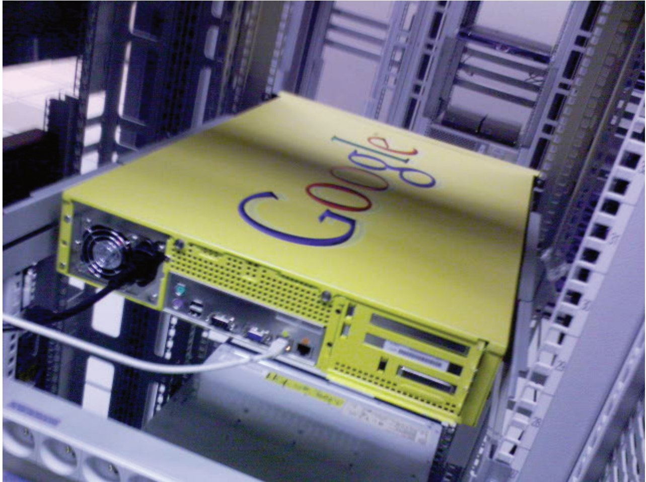
The Google Search Appliance is a hardware product that firms can purchase in order to run Google search technology within the privacy and security of an organization's firewall.
