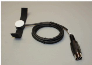
The PT-104 pulse plethysmograph.
