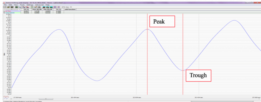
Methods Figure 4. Breathing pattern of a sitting subject displayed on the Lung Volumes channel in the Analysis window. The cursors are positioned on the peak of the breath cycle and the trough of the succeeding cycle to measure the maximum expiratory flow rate with the Min_dv/dt function.
