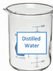
Figure 3. Rinse electrode with distilled water and place in beaker with enough clean distilled water to cover tip of electrode.
