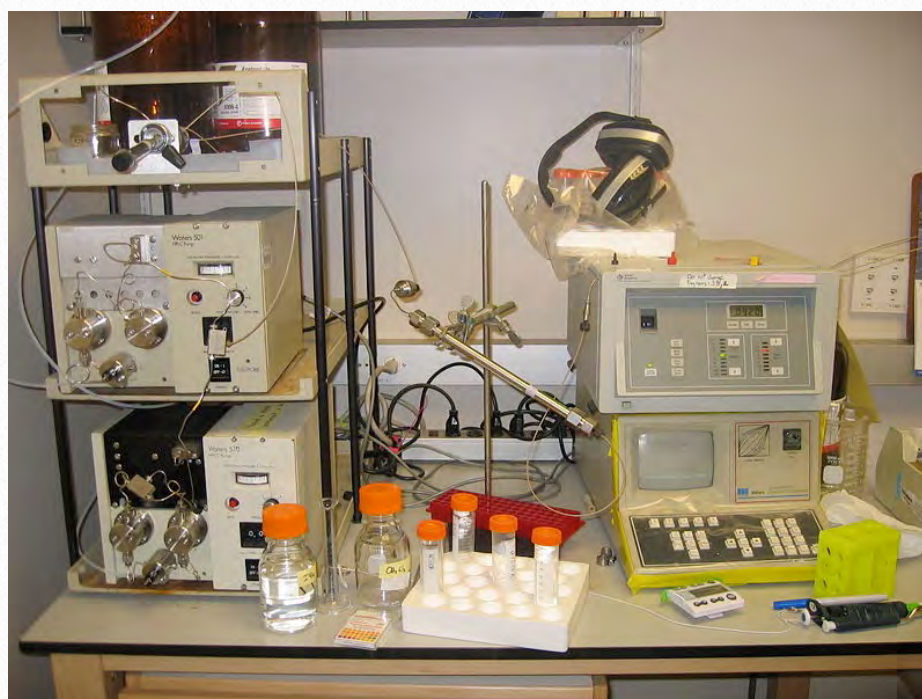
Figure 8.10 - HPLC: Pumps on left/Column in center/Detector on the right
