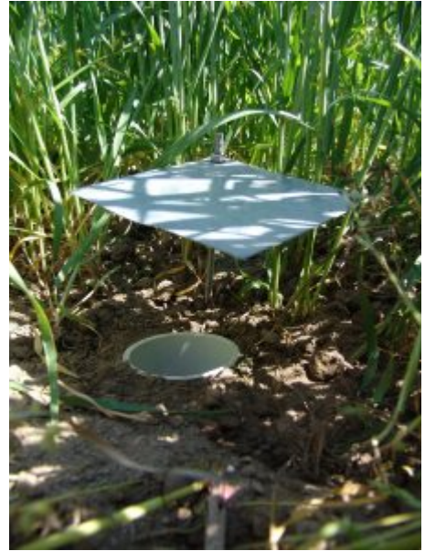
Figure 1-5: Pitfall traps are ideal for collection nocturnal and ground crawling species. Image source: https://commons.wikimedia.org/w/index.php?title=File:Barber_pitfall_trap.jpg&oldid=269026568
