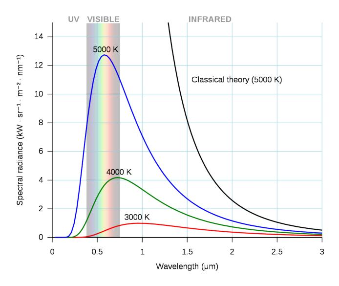
Figure 12: Example of three Planck curves, for surfaces at 3000-5000 degrees Kelvin. Black body by Darth Kule, Wikimedia Commons, public domain.
