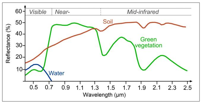
Figure 27: Spectral signatures of broadly defined common types of Earth surface materials. Reflectance of water, soil and vegetation at different wavelengths by Science Education through Earth Observation for High Schools (SEOS), CC BY-NC-SA 2.0.
