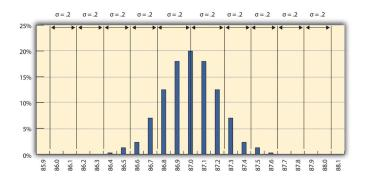
The refinery's quality control manager calculates that the new standard deviation is 0.2 octane. From this, he can use the 68-95-99.7 rule to estimate that 68.3% of the fuel produced will be between 86.8 and 87.2 and that 99.7% will be between 86.4 and 87.6 octane. A shorthand way of describing this amount of control is to say that it is a five-sigma production system, which refers to the five standard deviations between the mean and the control limit on each side.
