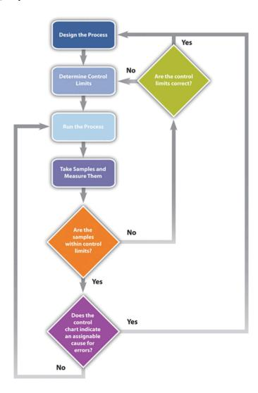
The process used to plan and assess **quality** can be described using flowcharts. They are useful for communicating processes that have logical branches that can be determined by simple yes or no questions. Flowcharting is also useful for discovering misunderstanding in project roles and responsibilities and communicating responsibility for work processes.
