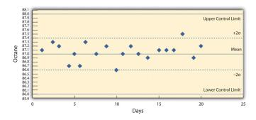
She recognizes that the highest and lowest measurements are not part of a trend and are probably due to chance causes. However, the control chart from the next twenty days, as shown below, indicates an upward trend that might be due to an **assignable cause**. She alerts the process manager to let him know that there is a problem that needs to be fixed before the product exceeds the upper control limit. This might indicate the need to initiate a project to fix the problem.
