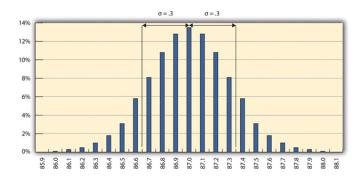
Most of the measurements are within 0.3 octane of 87.
