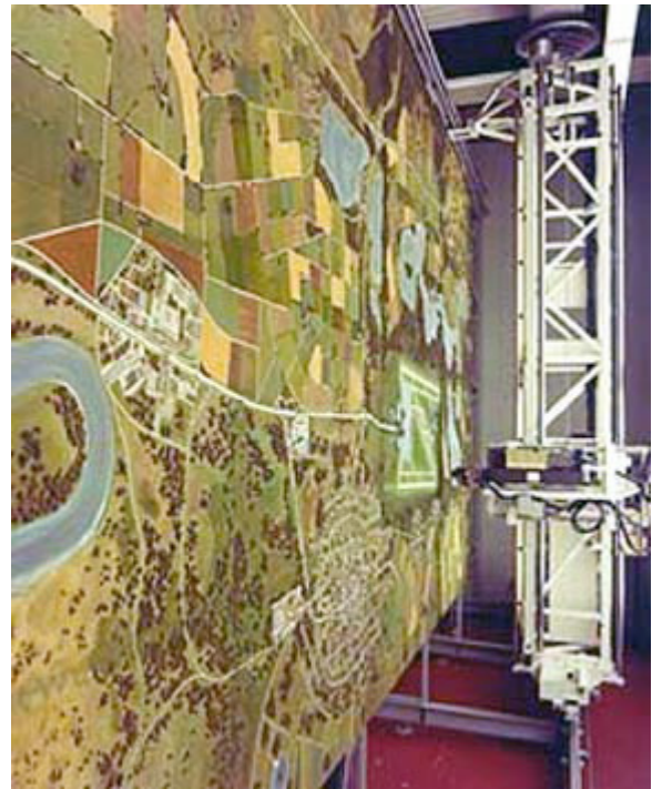
CCTV Terrain Board
