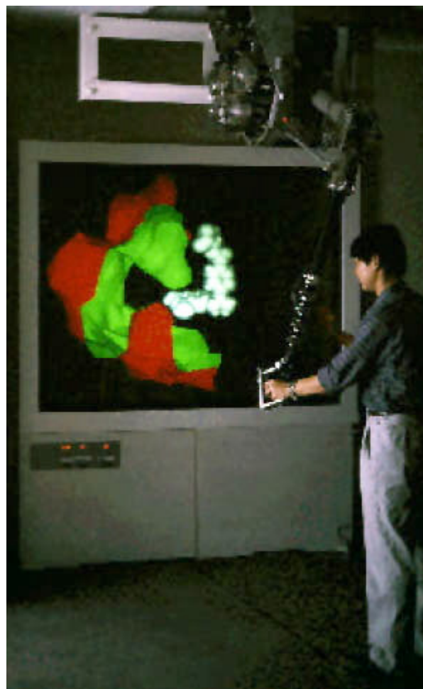
The Docker haptic feedback system
