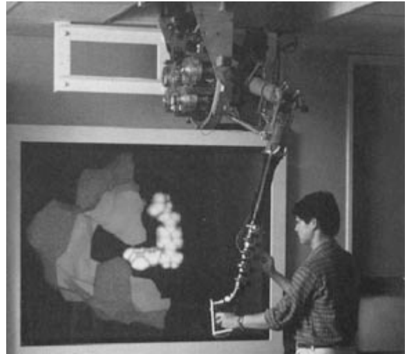
The Docker haptic feedback system
