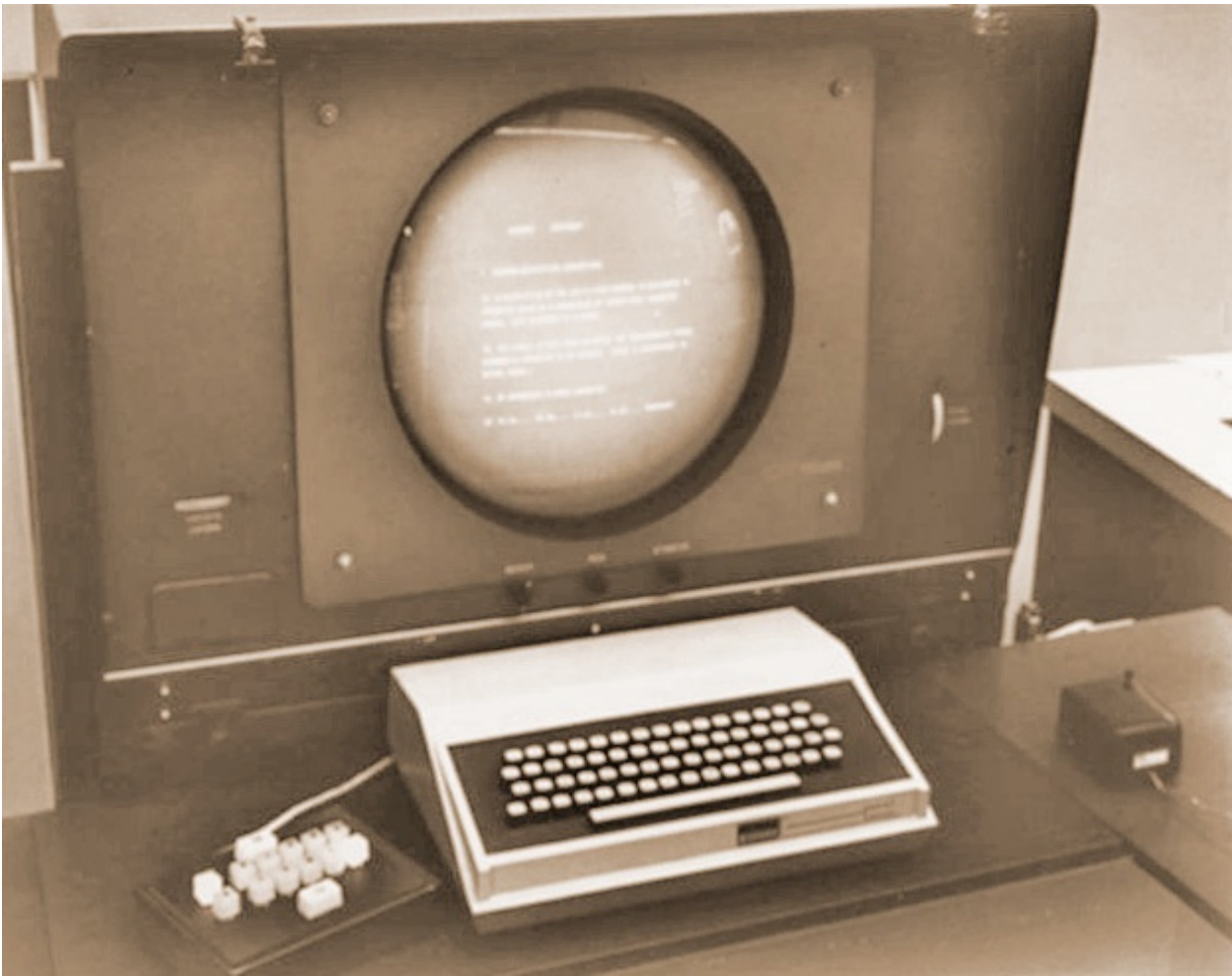
Engelbart's workstation, showing an early version (c1964) of the mouse
