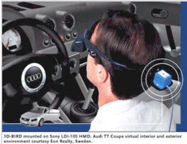
3D Bird mounted on the back of a Sony LDI-100 HMD in Audi TT coupe
