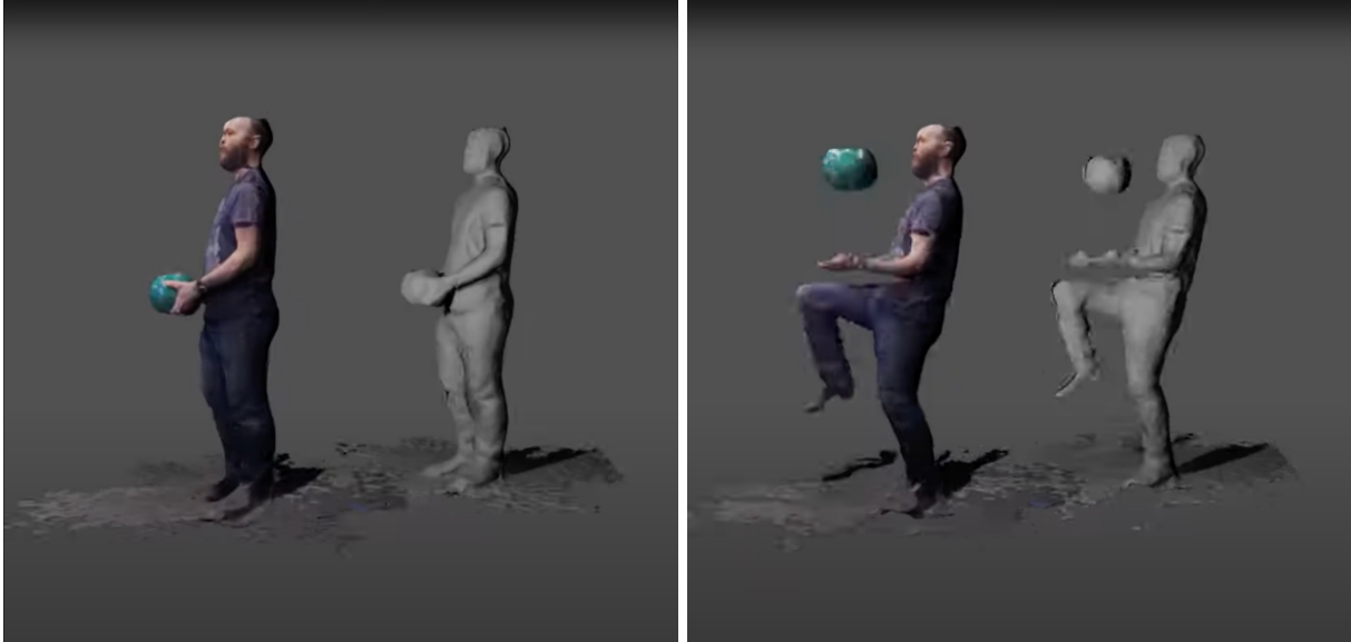
Figure 6: Point Cloud .ply sequence from LiveScan3D to Houdini. Houdini is used to mesh the point cloud sequence and you can see the resulting mesh both with colour and without.
