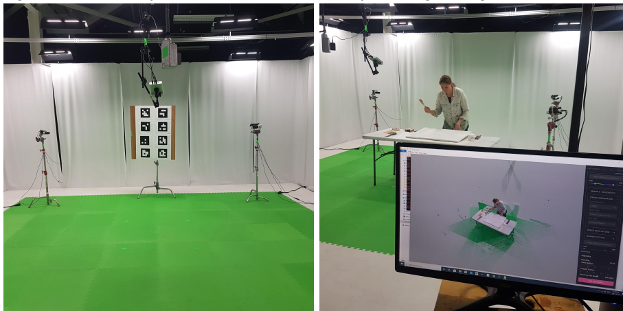
Figure 12: Left: Calibration target (calibration is done in pairs) Right: Live preview of point clouds
