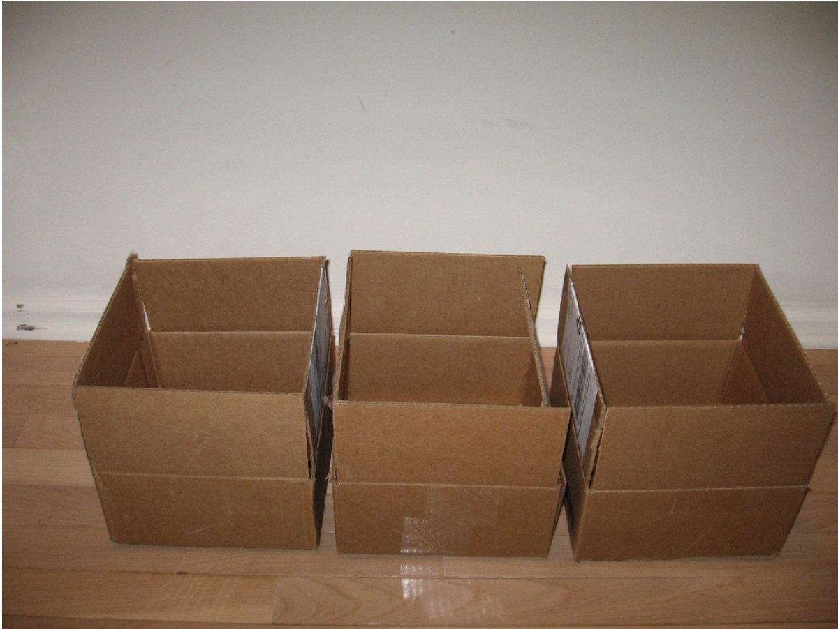
Figure 6.14: A single wholesale unit of a product, such as these empty cartons shown here, is an example of secondary packaging. Each of these boxes might hold, for example, twenty-four cans of car polish or thirty-six cans of bug spray.
