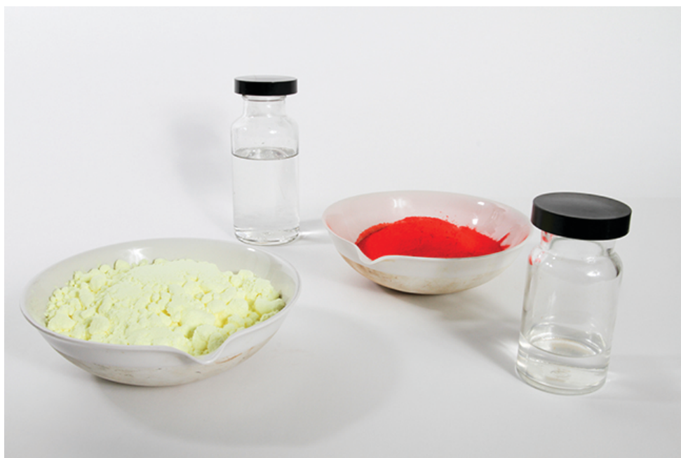
Figure 7.2c Each sample contains 6.02 \times 10^{23} molecules or formula units—1.00 mol of the compound or element. Clock-wise from the upper left: 130.2 g of C_8H_{17}OH (1-octanol, formula mass 130.2 amu), 454.4 g of HgI_2 (mercury(II) iodide, formula mass 454.4 amu), 32.0 g of CH_3OH (methanol, formula mass 32.0 amu) and 256.5 g of S_8 (sulfur, formula mass 256.5 amu). (credit: Sahar Atwa in Chemistry (OpenStax) , CC BY 4.0 ).
