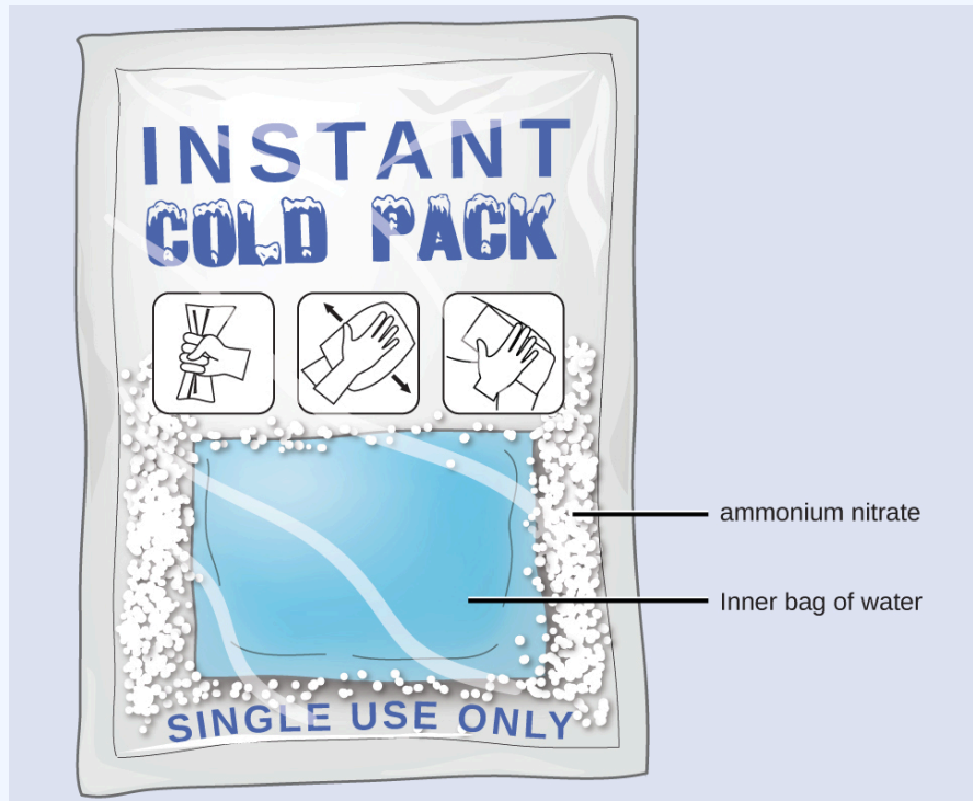
Figure 4.3e An instant cold pack consists of a bag containing solid ammonium nitrate and the second bag of water. When the bag of water is broken, the pack becomes cold because the dissolution of ammonium nitrate is an endothermic process that removes thermal energy from the water. The cold pack then removes thermal energy from your body (credit: Chemistry (OpenStax), CC BY 4.0 ).
