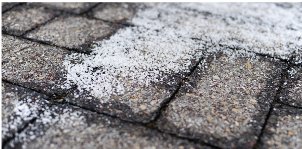
Figure 14.5d Rock salt (NaCl), calcium chloride (CaCl 2 ), or a mixture of the two are used to melt ice. (credit: modification of work by Eddie Welker, CC BY 2.0)
