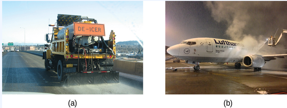
Figure 14.5e Freezing point depression is exploited to remove ice from (a) roadways and (b) the control surfaces of aircraft. (credit a: work by Oregon Department of Transportation, CC BY 2.0 ; credit b: work by Paolo Cerutti, CC BY 2.0 )
