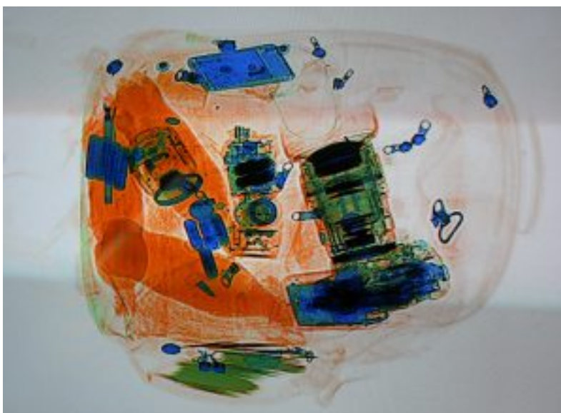
Figure 10.1h X-Ray Imaging for Security: This x-ray image shows the contents of a piece of luggage. The denser the material, the darker the shadow. (credit: work by IDuke , CC BY 2.5 )
