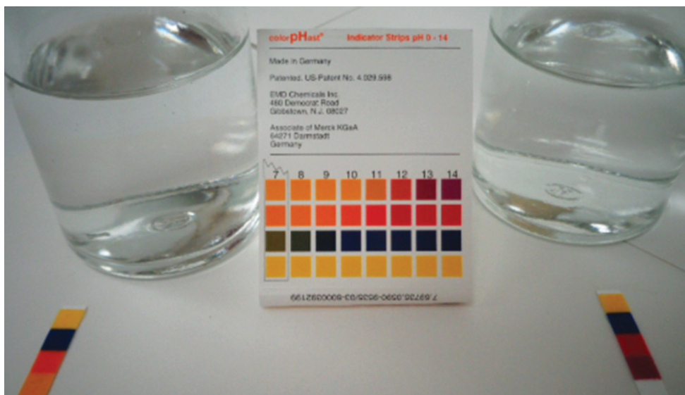
Figure 17.7e pH paper indicates that a 0.1- M solution of \text{NH}_3 (left) is weakly basic. The solution has a pOH of 3 ( [\text{OH}^-] = 0.001 \text{ M} ) because the weak base \text{NH}_3 only partially reacts with water. A 0.1- M solution of \text{NaOH} (right) has a pOH of 1 because \text{NaOH} is a strong base. (credit: modification of work by Sahar Atwa, Chemistry (OpenStax) , CC BY 4.0).
