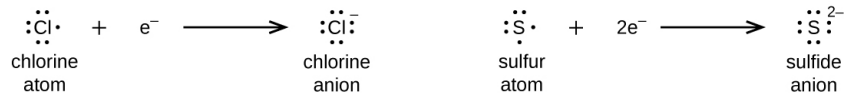
Figure 11.3e Formation of chloride and sulfide anions shown as Lewis structures (credit: Chemistry (OpenStax) , CC BY 4.0).
