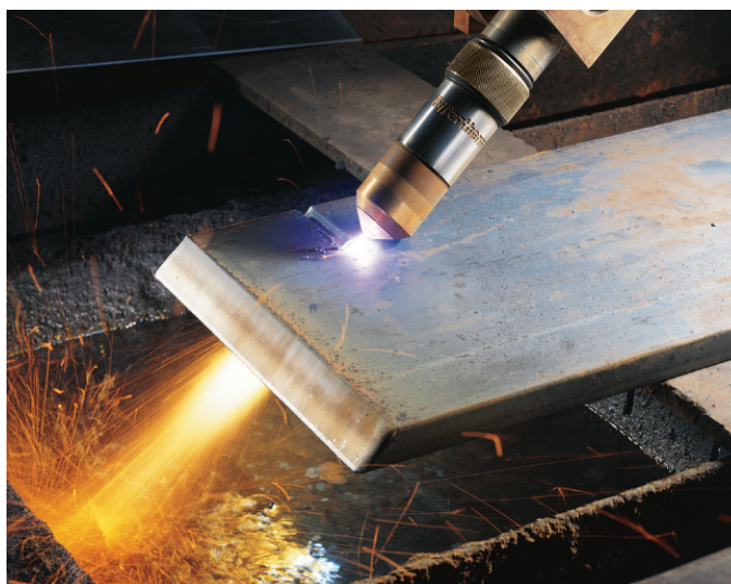
Figure 1.2c A plasma torch can be used to cut metal. (credit: work by Hypertherm, undeclared license)
