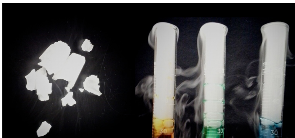
Figure 13a Solid carbon dioxide (“dry ice”, left) sublimates vigorously when placed in a liquid (right), cooling the liquid and generating a fog of condensed water vapour above the cylinder. (credit: modification of work by Paul Flowers in Chemistry (OpenStax) , CC BY 4.0).
