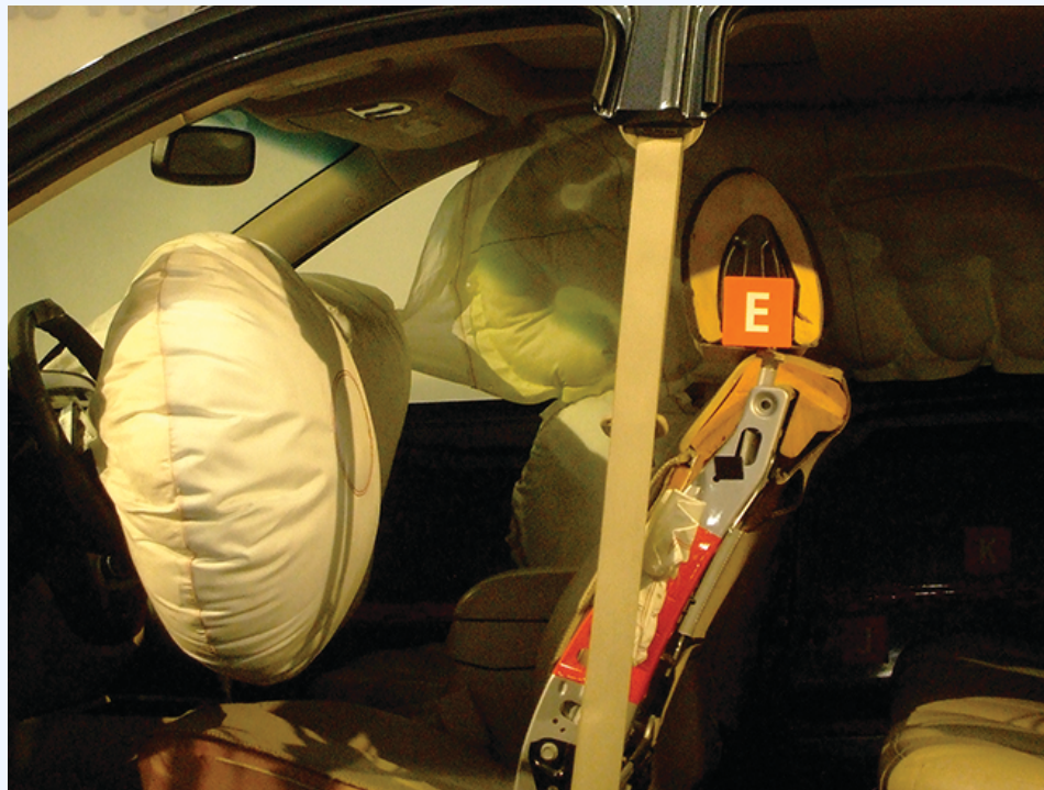
Figure 9.2b Airbags deploy upon impact to minimize serious injuries to passengers. (credit: work by Jon Seidman , CC BY 2.0 )
