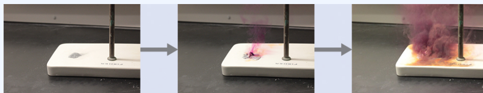
Figure 9.1a Aluminum and iodine react to produce aluminum iodide. The heat of the reaction vaporizes some of the solid iodine as a purple vapour. (credit: modification of work by Mark Ott in Chemistry (OpenStax) , CC BY 4.0).
