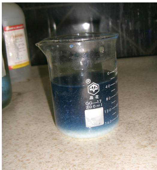
Figure 8.3b “Double-Replacement Reactions.” Some double-replacement reactions are obvious because you can see a solid precipitate coming out of the solution. (credit: work by Chojj, PD)
