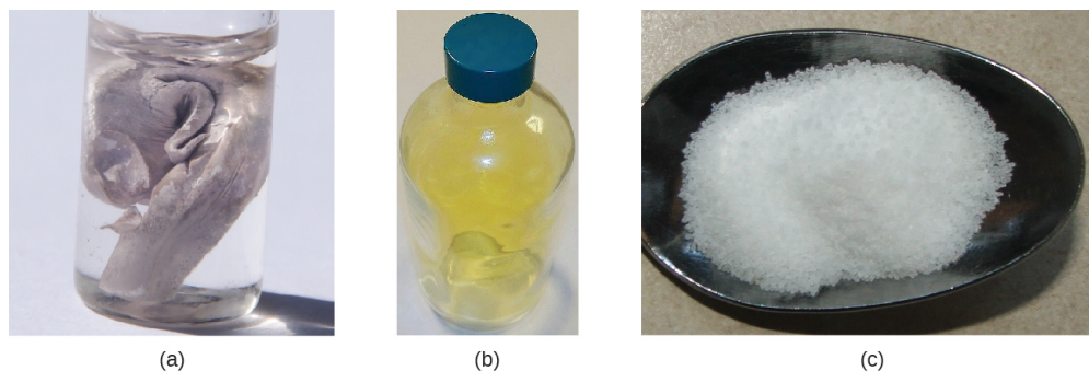
Figure 11.1a (a) Sodium is a soft metal that must be stored in mineral oil to prevent reaction with air or water. (b) Chlorine is a pale yellow-green gas. (c) When combined, they form white crystals of sodium chloride (table salt). (credit a: modification of work by Jurii , CC BY 3.0 ; b: work by Greenhorn1 , PD ; c: work by Chemicalinterest , PD )
