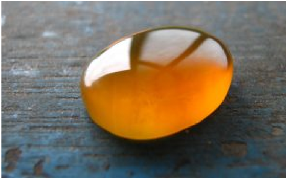
Figure 5.2c Image of Borneo Amber: Borneo amber is mined in Sabah, Malaysia, from shale-sandstone-mudstone veins. When a piece of amber is rubbed with a piece of fur, the amber gains more negative charge, giving it a net negative charge. At the same time, the fur, having lost what we now know to be called electrons, becomes positively charged. (credit: work by Sebakoamber, PD )
