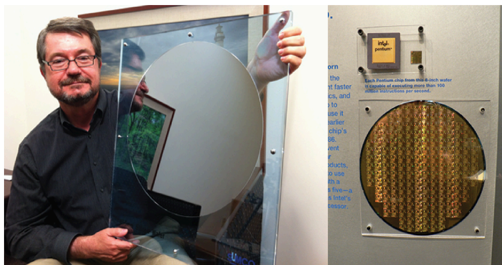
Figure 3a Purity is extremely important when preparing silicon wafers. The CEO of VLSI Research, Don Hutcheson, shows off a pure silicon wafer (left). A silicon wafer covered in Pentium chips is an enlarged version of the silicon wafers found in many electronics used today (right). (credit left: modification of work by Intel Free Press, CC BY 2.0; credit right: modification of work by Naotake Murayama ( https://www.flickr.com/people/12832970@N00 ), CC BY 2.0)
