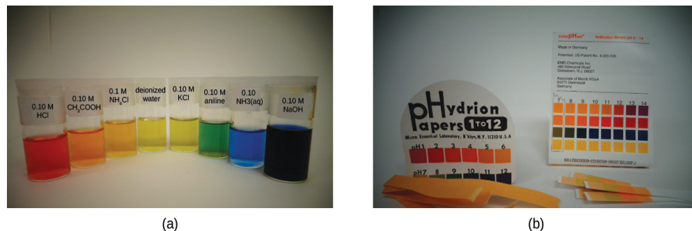
Figure 16.4c (a) A universal indicator assumes a different colour in solutions of different pH values. Thus, it can be added to a solution to determine the pH of the solution. The eight vials each contain a universal indicator and 0.1-M solutions of progressively weaker acids: HCl (pH = 1), CH 3 CO 2 H (pH = 3), and NH 4 Cl (pH = 5), deionized water, a neutral substance (pH = 7); and 0.1-M solutions of the progressively stronger bases: KCl (pH = 7), aniline, C 6 H 5 NH 2 (pH = 9), NH 3 (pH = 11), and NaOH (pH = 13). (b) pH paper contains a mixture of indicators that give different colours in solutions of differing pH values. (credit: modification of work by Sahar Atwa in Chemistry (OpenStax) , CC BY 4.0).
