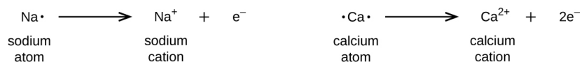
Figure 11.3d Formation of sodium and calcium cations shown as Lewis structures (credit: Chemistry (OpenStax) , CC BY 4.0).
