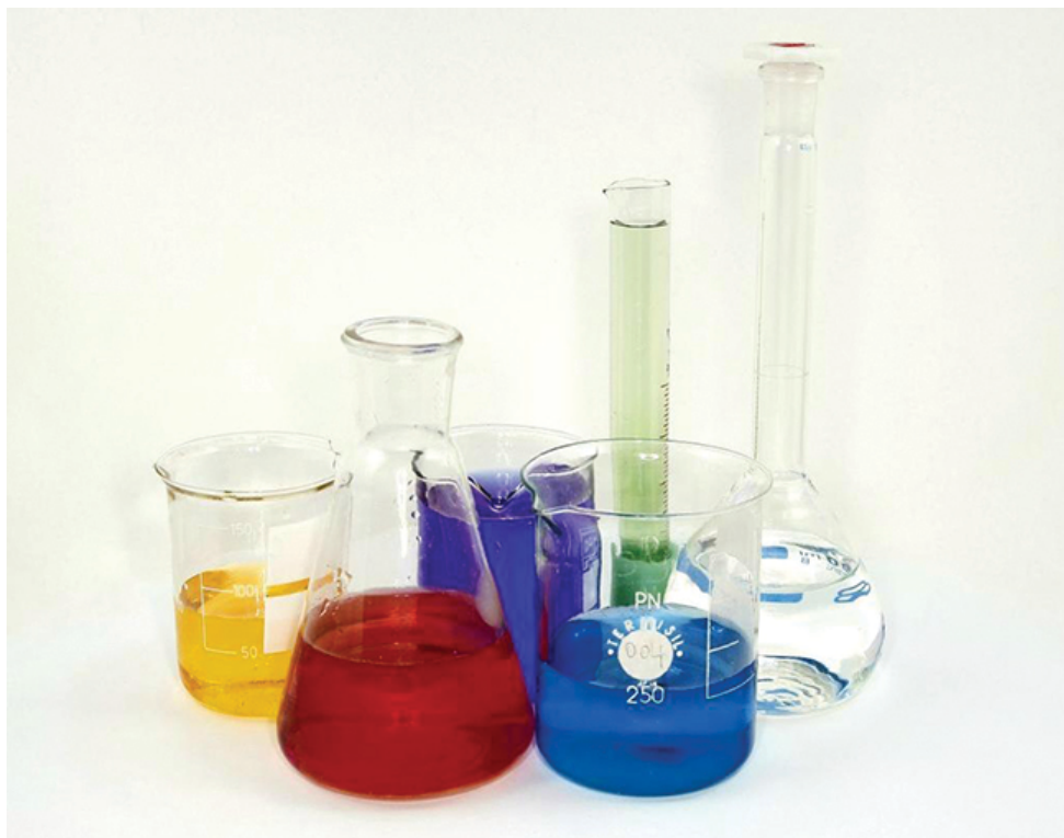
Figure 3.2e Laboratory glassware, such as Pyrex and Kimax, is made of borosilicate glass because it does not break when heated. The inclusion of borates in the glass helps to mediate the effects of thermal expansion and contraction. This reduces the likelihood of thermal shock, which causes silicate glass to crack upon rapid heating or cooling. (credit: photo by Tweenk, CC BY 3.0)
