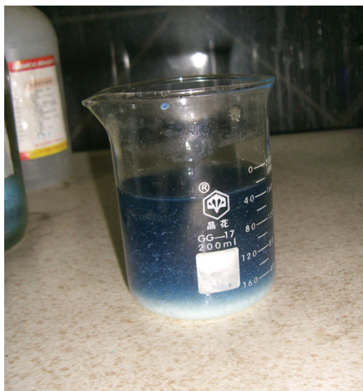
Figure 8.3b “Double-Replacement Reactions.” Some double-replacement reactions are obvious because you can see a solid precipitate coming out of the solution. (credit: work by Choij, PD)
