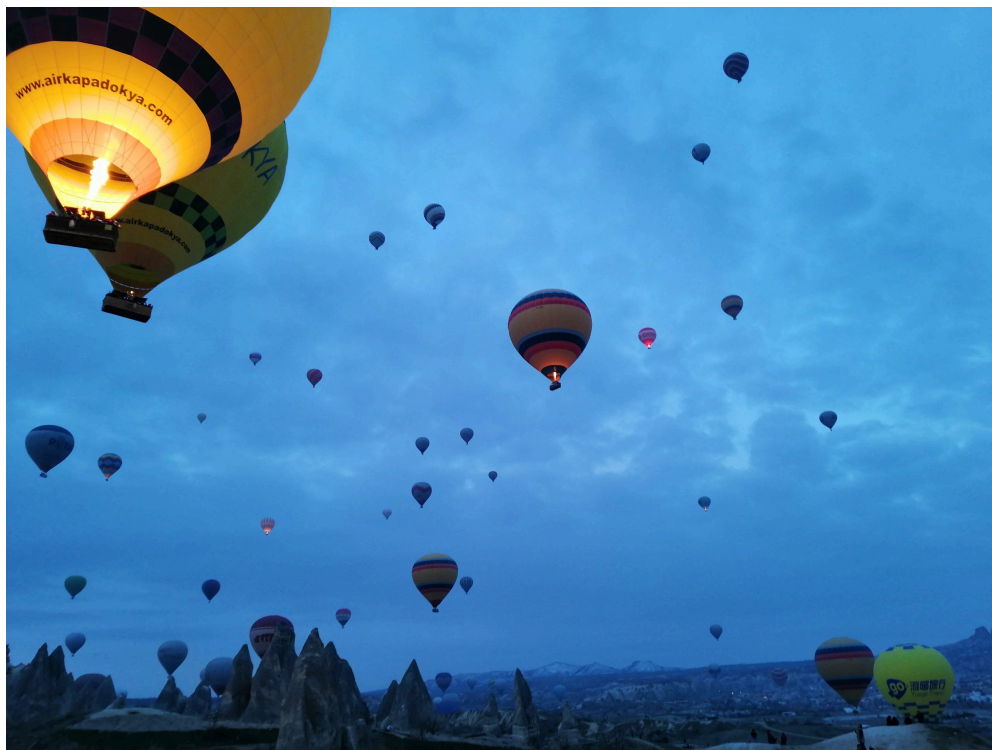
Figure 12a The hot air inside these balloons is less dense than the surrounding cool air. This results in a buoyant force that causes the balloons to rise when their guy lines are untied. (credit: work by Elif Tütüncü, CC BY-SA 4.0)
