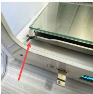
The photo shows the clamps that keep the build plate glass in place. Photo: Hanne Pearce
