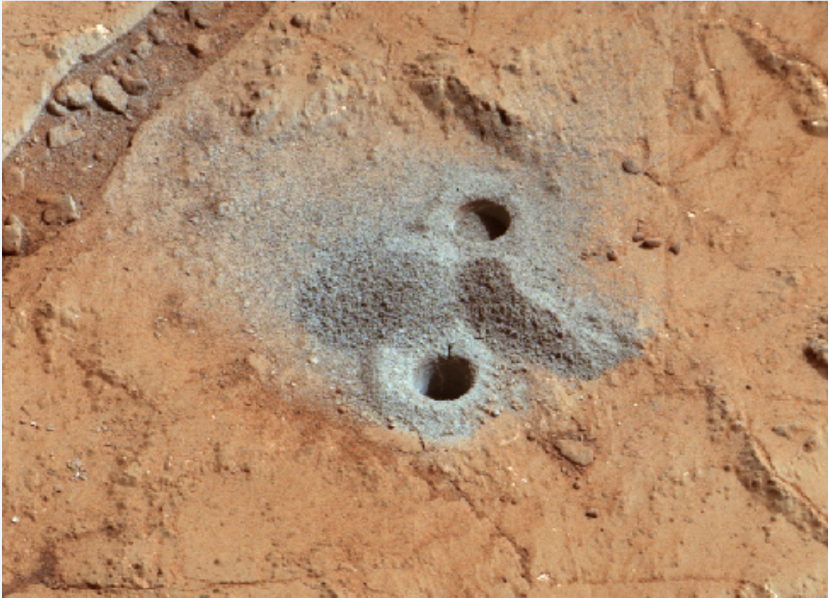
Figure 16.11. Shown are the first holes drilled by NASA's Curiosity Mars rover into a mudstone, with "fresh" drill-pilings around the holes. Notice the difference in colour between the red ancient martian surface and the grey newly exposed rock powder that came from the drill holes. Each drill hole is about 0.6 inch (1.6 cm) in diameter. (credit: modification of work by NASA/JPL-Caltech/MSSS) Dust from Mars Drilling: Tailings and Discard Piles by NASA, NASA/JPL Image Use Policy.
