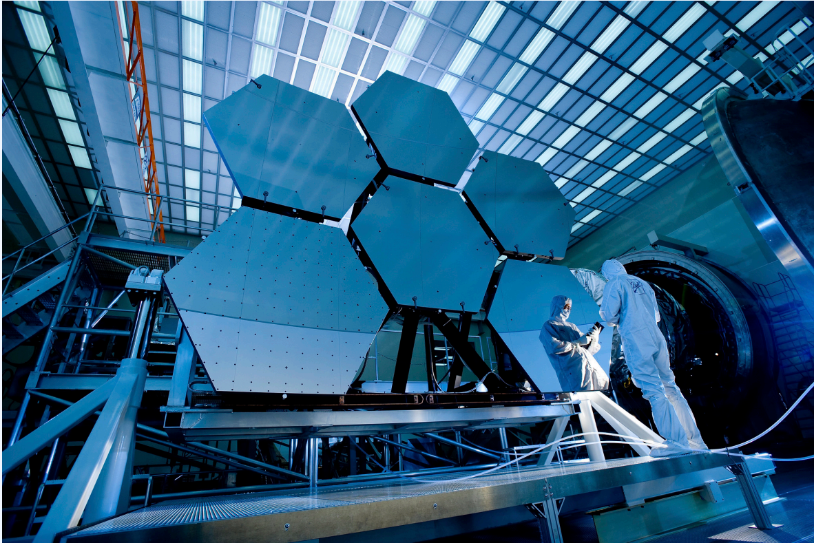
Figure 4.30. This image shows some of the mirrors of the JWST as they underwent cryogenic testing. The mirrors were exposed to extreme temperatures in order to gather accurate measurements on changes in their shape as they heated and cooled.
