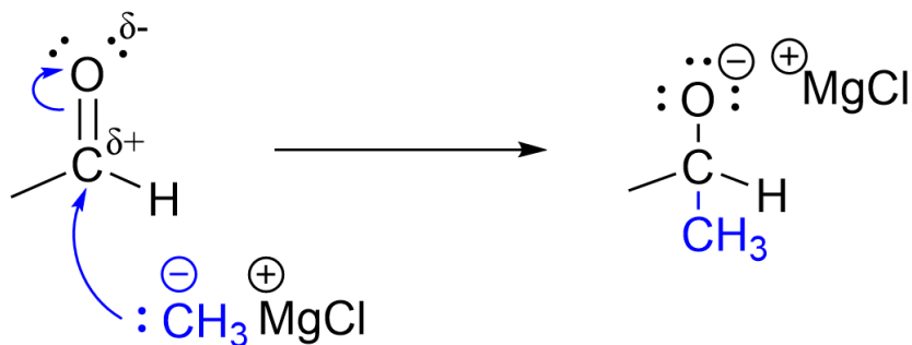
Figure 3.4.2.e. The first step in the Grignard reaction with an aldehyde. In this step, the Grignard reagent, which contains a nucleophilic carbon, attacks the electrophilic carbon carbonyl center, breaking the C=O \pi bond.
