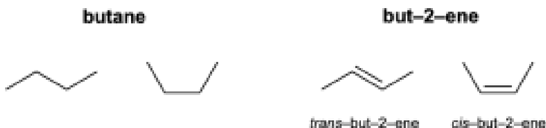
Figure 2.5.1.a. The two structures on the left represent the different conformations of butane, as alkanes experience free rotation. The two structures on the right represent the two configurations of but-2-ene: trans -but-2-ene and cis -but-2-ene.
