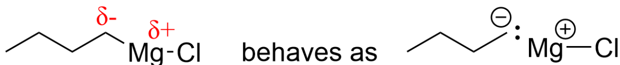
Figure 3.4.2.c. The R-MgX Grignard reagent contains a carbon atom with a partial negative charge, which can also be depicted as a lone pair of electrons and a formal negative charge on carbon. The carbon atom acts as a nucleophile.
