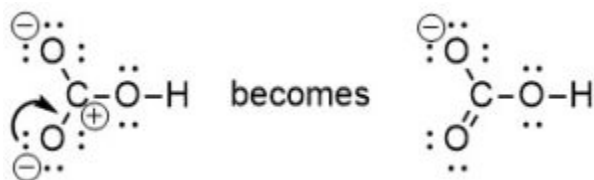
Figure 2.1.e. Minimize non-zero formal charge by sharing a lone pair of electrons between the bottom left oxygen atom and the central carbon atom. This generates a double bond between C and O.
