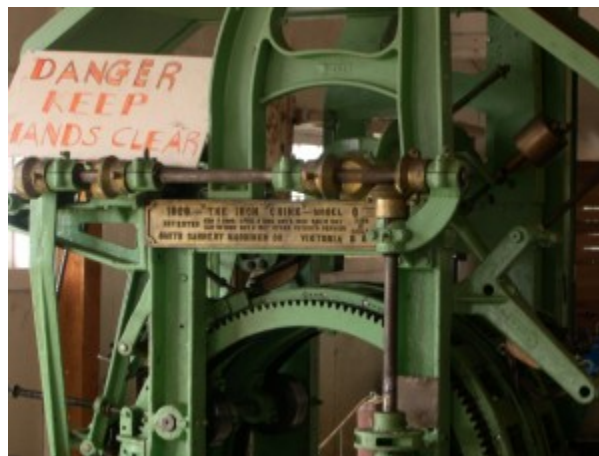
Figure 3.17 It would be difficult not to be simultaneously impressed by innovative machinery like this one and concerned about the displacement of labour that it entailed. The “Iron Chink” revolutionized the salmon canning industry on the Pacific Northwest coast.
