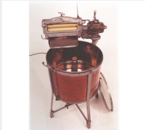
Figure 8.23 A pre-WWII washing machine produced by Beatty Brothers. Note the wringer – or mangle – in which children’s fingers are going to get squished.
