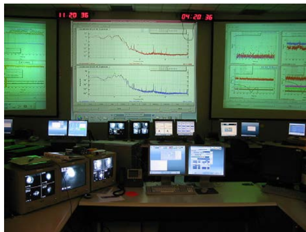
Figure 34.15 The control room of the LIGO gravitational wave detector. Gravitational waves will cause extremely small vibrations in a mass in this detector, which will be detected by laser interferometer techniques. Such detection in coincidence with other detectors and with astronomical events, such as supernovas, would provide direct evidence of gravitational waves. (credit: Tobin Fricke)
