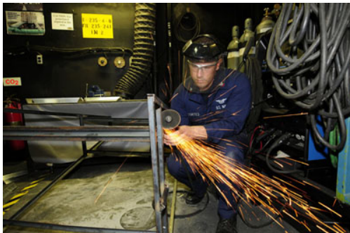
Figure 10.14 The motor works in spinning the grindstone, giving it rotational kinetic energy. That energy is then converted to heat, light, sound, and vibration. (credit: U.S. Navy photo by Mass Communication Specialist Seaman Zachary David Bell)
