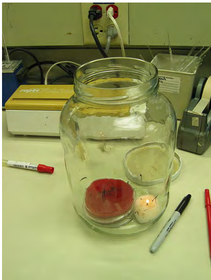
Figure 4.3 Candle Jar . Anaerobiosis is produced by a sealed jar and a candle inside, so microorganisms in the culture plates can survive and grow. The candle is lit, chamber sealed and when the candle is extinguished, the oxygen in the jar is reduced.
