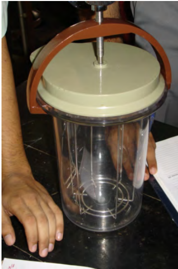
Figure 4.4 Gas-Pak jar. Gas-pak is a method used in production of an anaerobic environment. It is used to culture bacteria which die or fail to grow in presence of oxygen.
