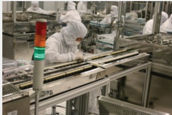
Figure 4.18. Assembly of notebook hard drives in Seagate’s “clean room.” Wuxi China (Photo courtesy of Robert Scoble/ Twitter)
