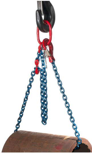
Figure 7 — Chain hook secured to master ring
