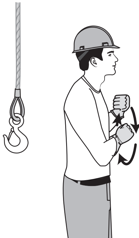
Figure 20—Crawler travel, both tracks
