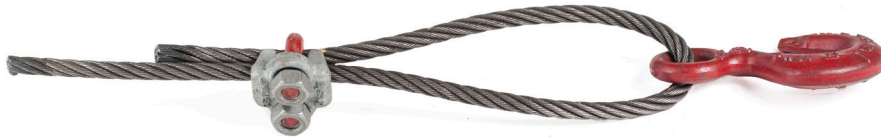
Figure 25 — Installing first cable clip
