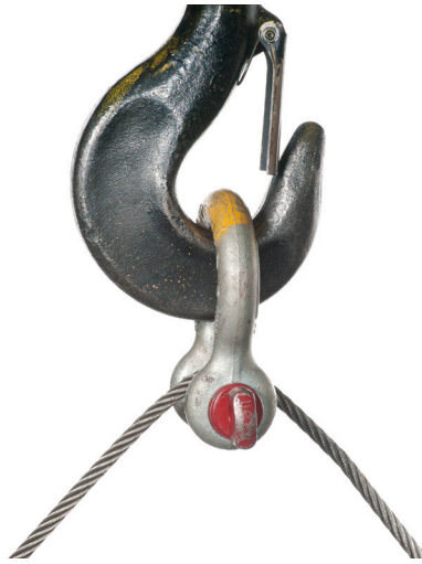
Figure 21 — Incorrect shackle attachment
