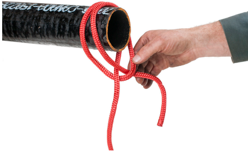
Figure 17 — Clove hitch pre-tied to slip over end of pipe
