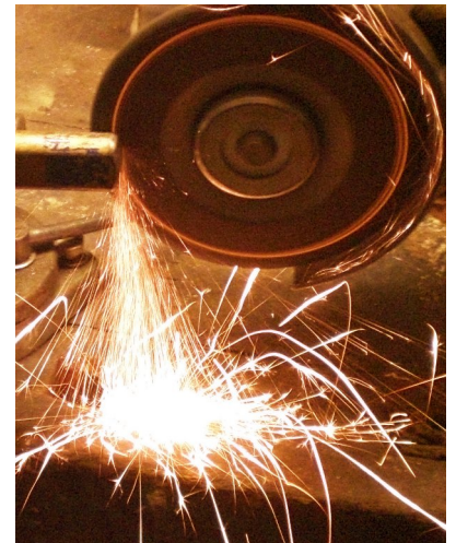
d / Sparks fly away along tangents to a grinding wheel.
