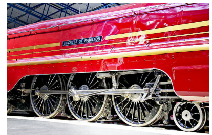
d / The locomotive’s wheels spin at a frequency of f cycles per second, which can also be described as \omega radians per second. The mechanical linkages allow the linear vibration of the steam engine’s pistons, at frequency f , to drive the wheels.
