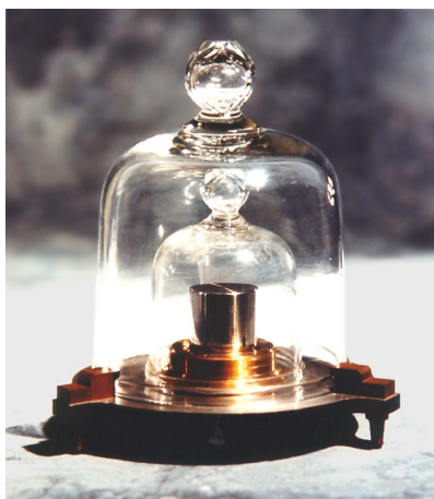
f/A duplicate of the Paris kilogram, maintained at the Danish National Metrology Institute.
