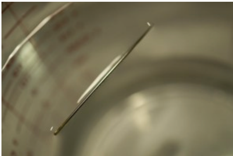
Figure 2.10 The weight of a needle on top of water pulls the surface tension downward; at the same time, the surface tension of the water is pulling it up, suspending the needle on the surface of the water and keeping it from sinking. Notice the indentation in the water around the needle. (credit: Cory Zanker)
