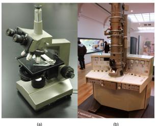
**Figure 4.2** (a) Most light microscopes used in a college biology lab can magnify cells up to approximately 400 times and have a resolution of about 200 nanometers. (b) Electron microscopes provide a much higher magnification, 100,000x, and a have a resolution of 50 picometers. (credit a: modification of work by "GcG"/Wikimedia Commons; credit b: modification of work by Evan Bench)
