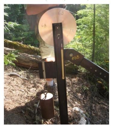
Figure 15.19 Part of a motion-monitoring device at the Checkerboard Slide near Revelstoke, B.C. The lower end of the cable is attached to a block of rock that is unstable. Any incremental motion of that block will move the cable, which will be detectable on this device. [SE]
