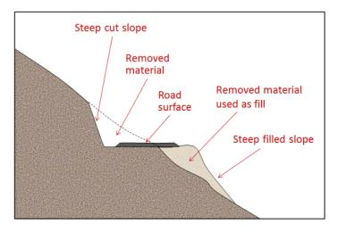
Figure 15.18 An example of a road constructed by cutting into a steep slope and the use of the cut material as fill. [SE]
