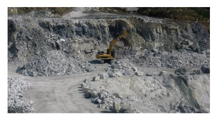
Figure 20.16 Triassic Quatsino Formation limestone being quarried on Texada Island, B.C. [SE]
