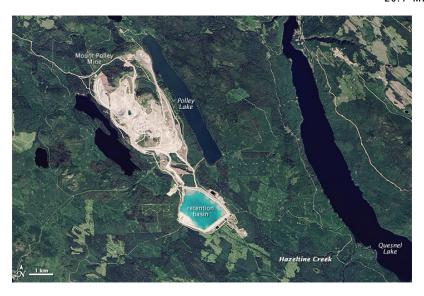
Figure 20.14a The Mt. Polley Mine area prior to the dam breach of August 2014. The tailings were stored in the area labelled "retention basin." [https://en.wikipedia.org/wiki/Mount\_Polley\_mine\_disaster]
