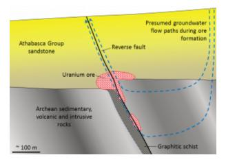
Figure 20.8 Model of the formation of unconformity-type uranium deposits of the Athabasca Basin, Saskatchewan [SE]
