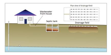
Figure 14.25 A typical septic system. [SE]
