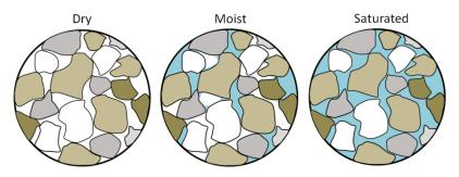
Figure 15.5 Depiction of dry, moist, and saturated sand [SE]
