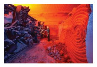
Figure 6.16 A mining machine at the face of potash ore (sylvite) in the Lanigan Mine near Saskatoon, Saskatchewan. The mineable potash layer is about 3 m thick.
