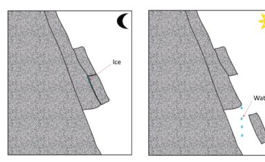
Figure 15.7 The contribution of freeze-thaw to rock fall [SE]
