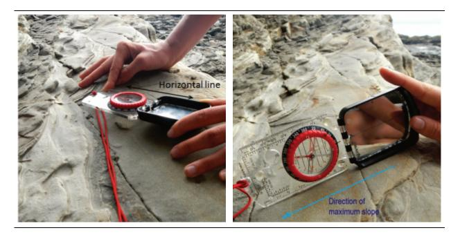
Figure 12.19 Measurement of strike (left) and dip (right) using a geological compass with a clinometer. [SE]
