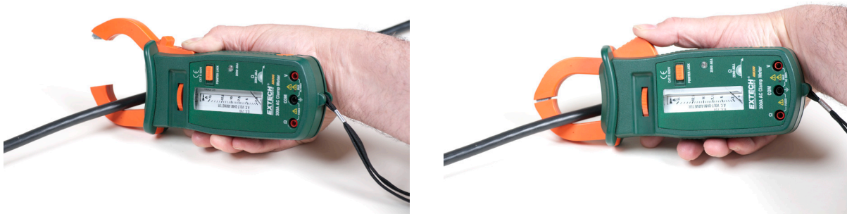
Figure 7 — Using clamp-on ammeter
