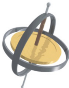
Figure 11.19 A gyroscope consists of a spinning disk about an axis that is free to assume any orientation.
