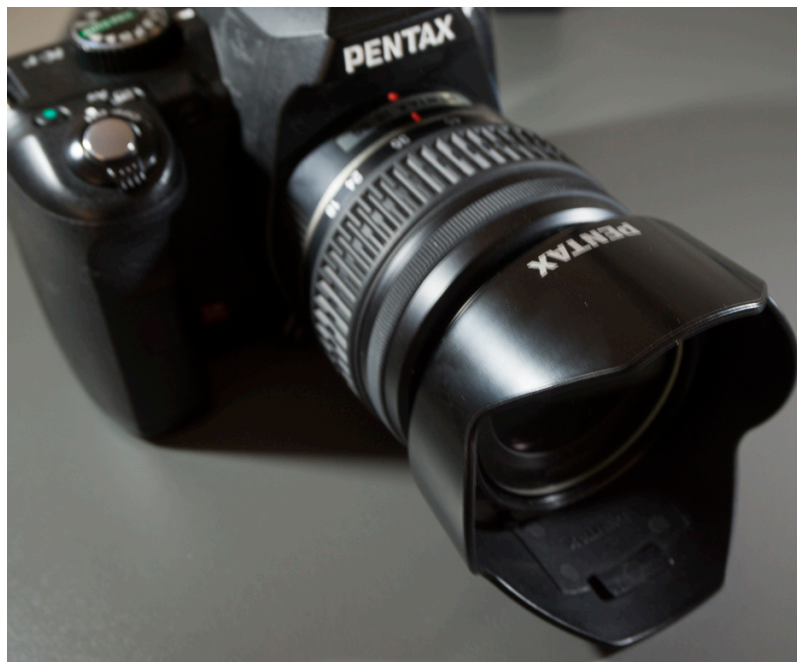
Figure 14-14. A lens hood reduces reflected glare onto the lens, which increases the contrast of photos and avoids artifacts from stray light. Photo Richard Adams. Image licensed under CC BY 4.0.
