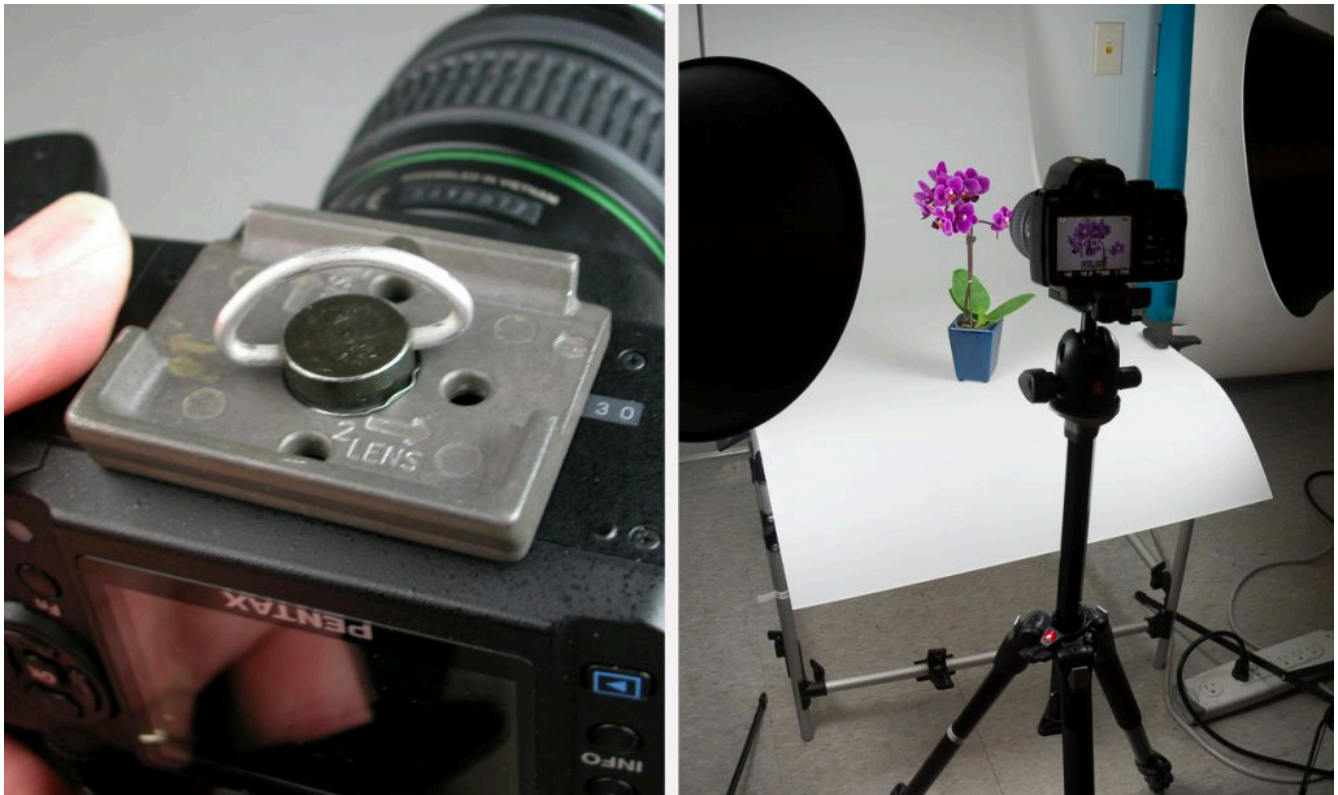
Figure 14-5. Quick-release tripod mount includes a plate that screws into the camera mount and then clips onto the tripod, allowing for rapid on-and-off operation. Photos Richard Adams. Image licensed under CC BY 4.0.
