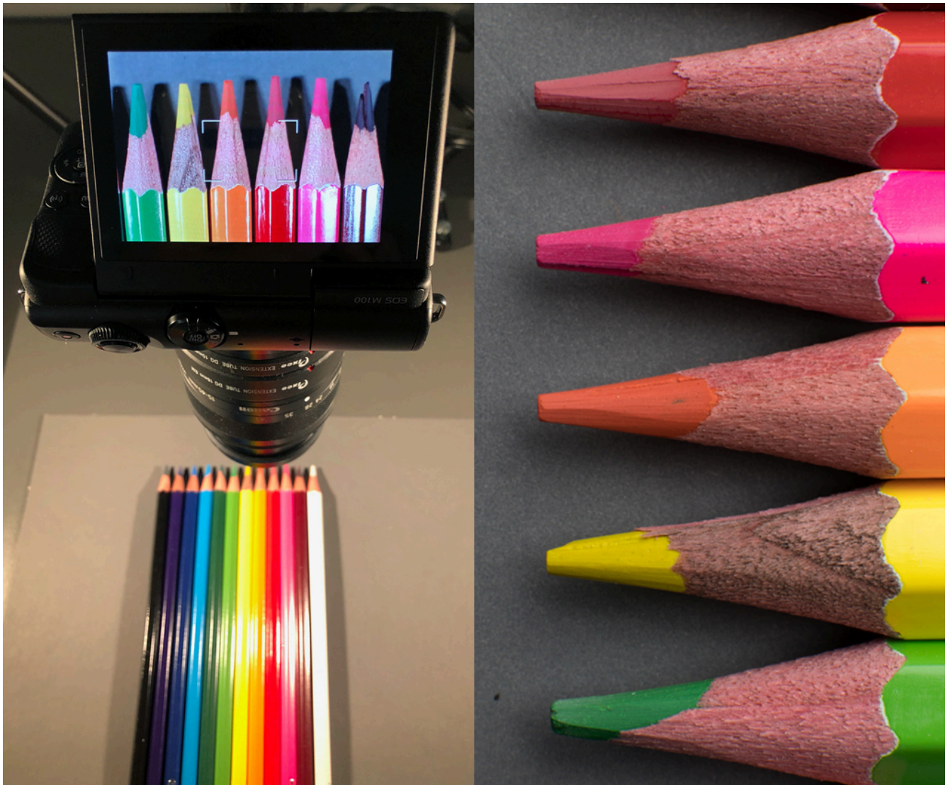
Figure 14-15. A macro lens (left) is useful for photographing items up close, typically with a 1:1 reproduction ratio, so the item is captured in its actual size (right) on the sensor. Photos Richard Adams. Image licensed under CC BY 4.0.
