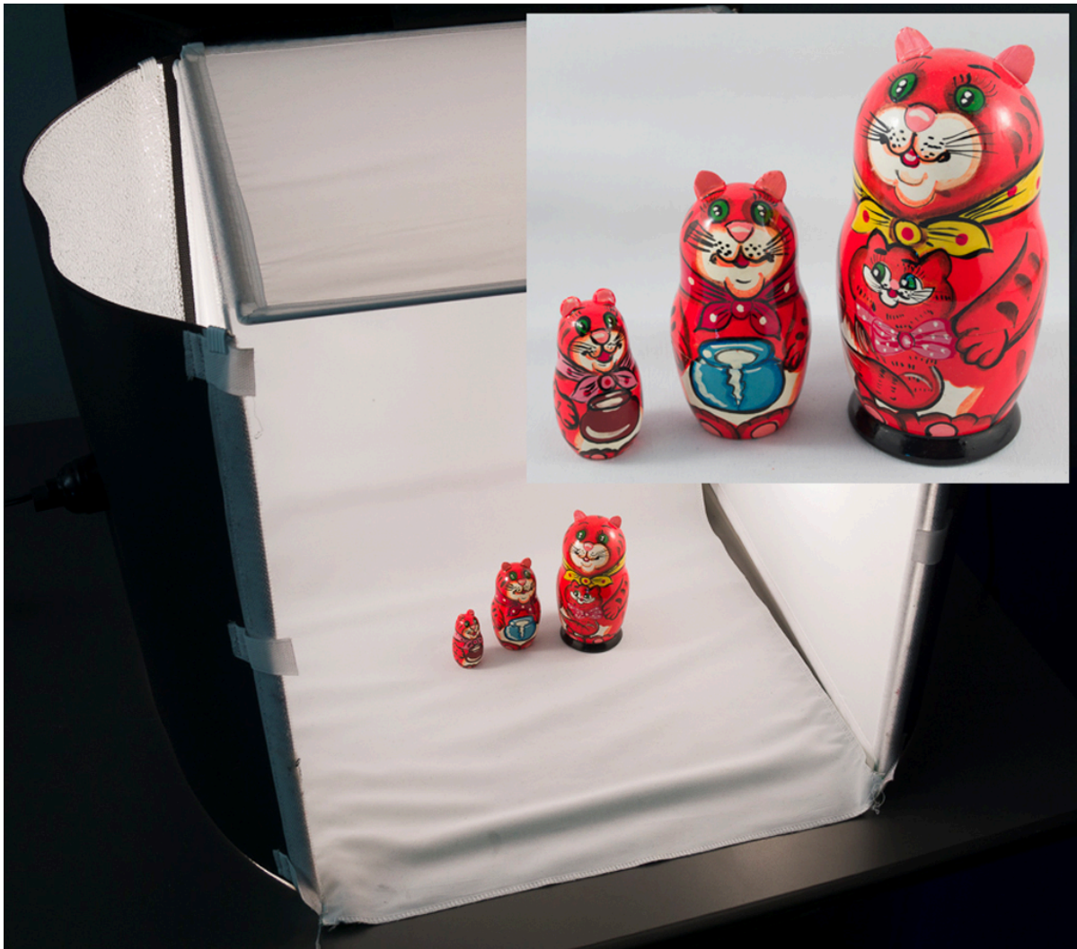
Figure 14-12. A light tent provides diffuse light for product photography. Photo Richard Adams. Image licensed under CC BY 4.0.
