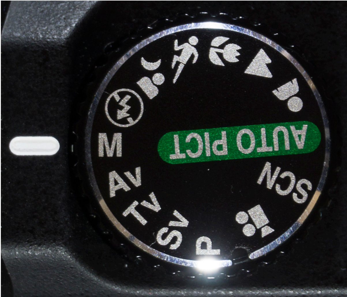
Figure 14-2. Mode dial on a DSLR camera includes manual, aperture priority (“Av”), shutter priority (“Tv”), ISO priority (“Sv”), and program (“P”) modes, along with various scene settings. For web work manual gives the greatest control and consistency. Photo Richard Adams. Image licensed under CC BY 4.0.
