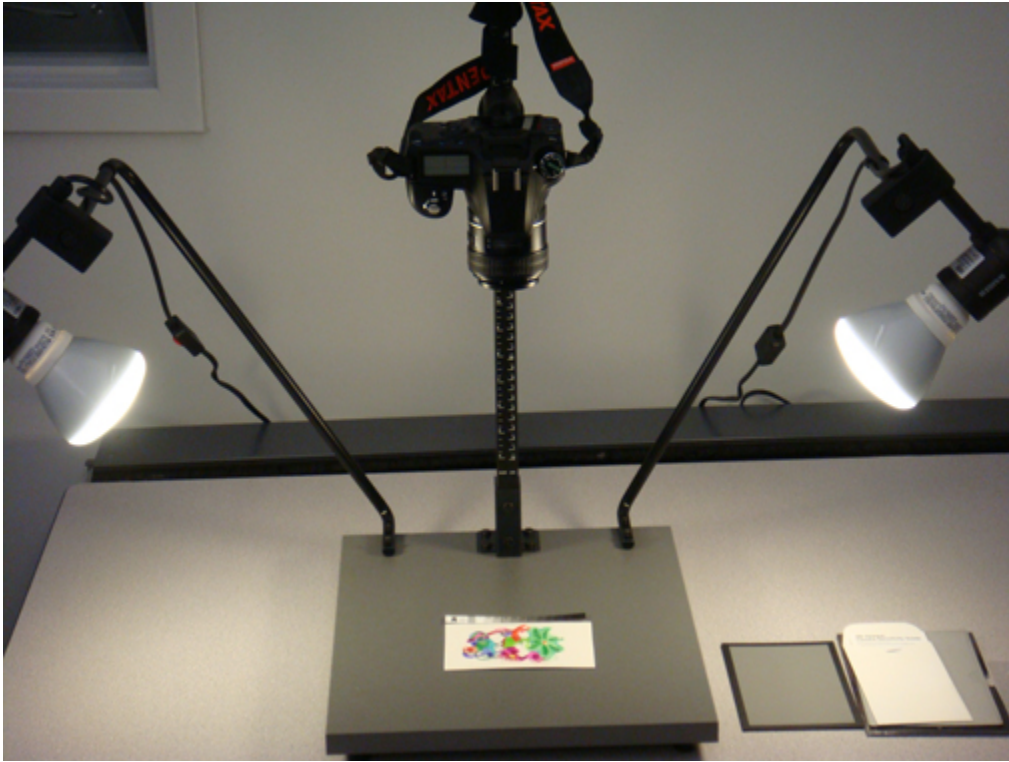
Figure 14-3. A 15% grey card (to right of table) is used to set manual exposure to 0 EV on this DSLR copy stand setup. Photo Richard Adams. Image licensed under CC BY 4.0.
