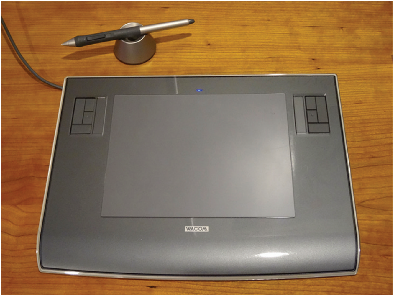
Figure 10.7.1 A tablet with a specially designed pen to write with is another application of magnetic induction.
