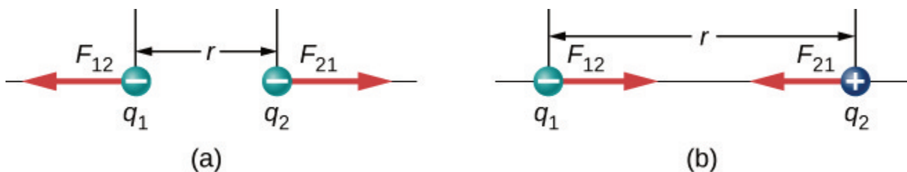
Figure 1.3.1. The electrostatic force \vec{\mathbf{F}} between point charges q_1 and q_2 separated by a distance r is given by Coulomb's law. Note that Newton's third law (every force exerted creates an equal and opposite force) applies as usual—the force on q_1 is equal in magnitude and opposite in direction to the force it exerts on q_2 . (a) Like charges; (b) unlike charges.
