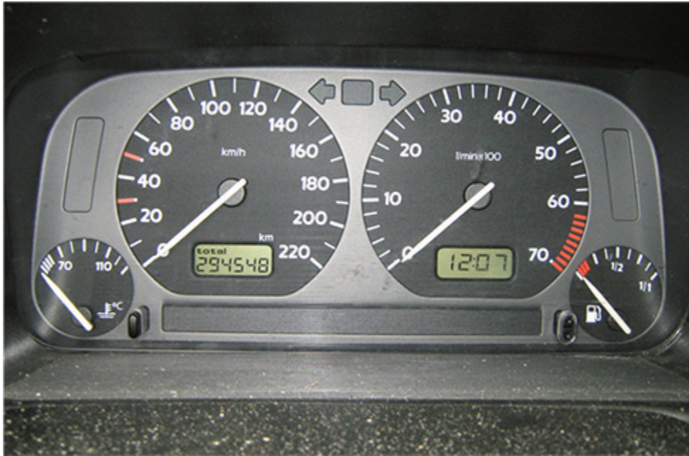
Figure 6.4.1 The fuel and temperature gauges (far right and far left, respectively) in this 1996 Volkswagen are voltmeters that register the voltage output of “sender” units. These units are proportional to the amount of gasoline in the tank and to the engine temperature. (credit: Christian Giersing)
