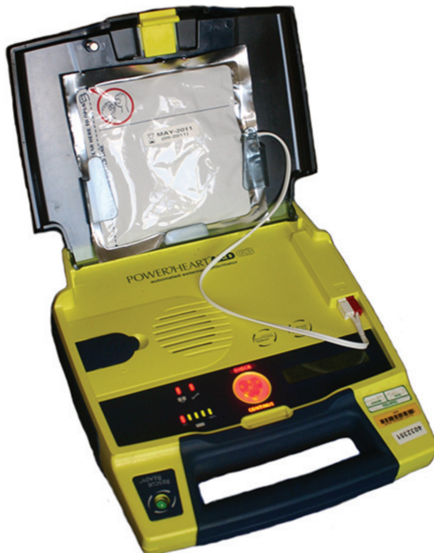
Figure 4.3.2 Automated external defibrillators are found in many public places. These portable units provide verbal instructions for use in the important first few minutes for a person suffering a cardiac attack.
