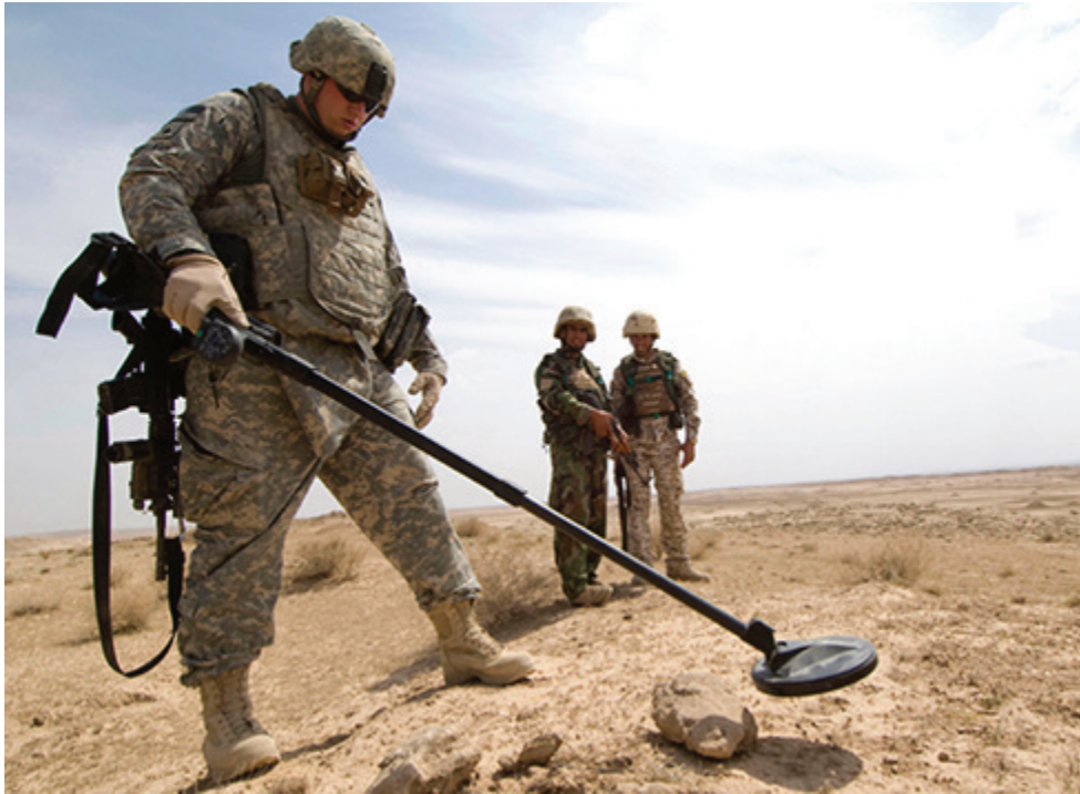
Figure 10.5.6 A soldier in Iraq uses a metal detector to search for explosives and weapons. (credit: U.S. Army)
