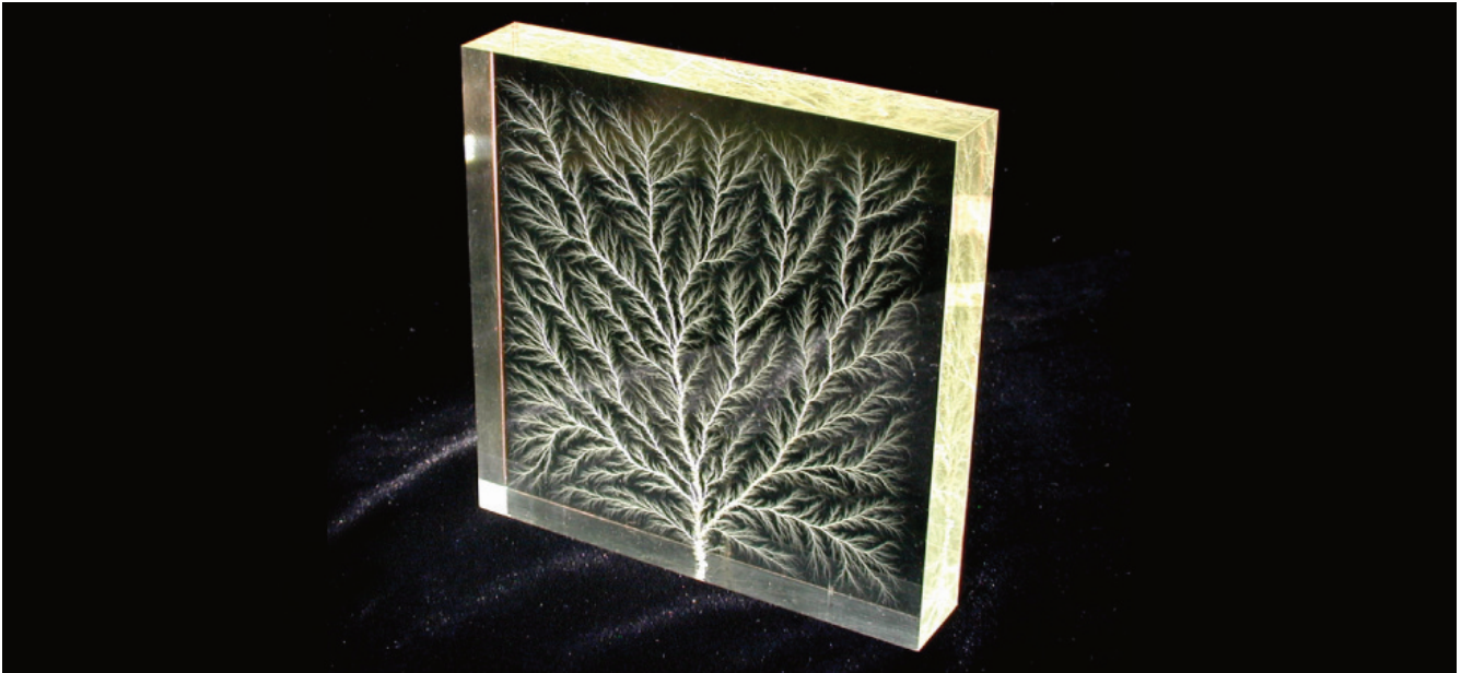
Figure 4.0.1. The tree-like branch patterns in this clear Plexiglas® block are known as a Lichtenberg figure, named for the German physicist Georg Christof Lichtenberg (1742–1799), who was the first to study these patterns. The “branches” are created by the dielectric breakdown produced by a strong electric field. (credit: modification of work by Bert Hickman)
