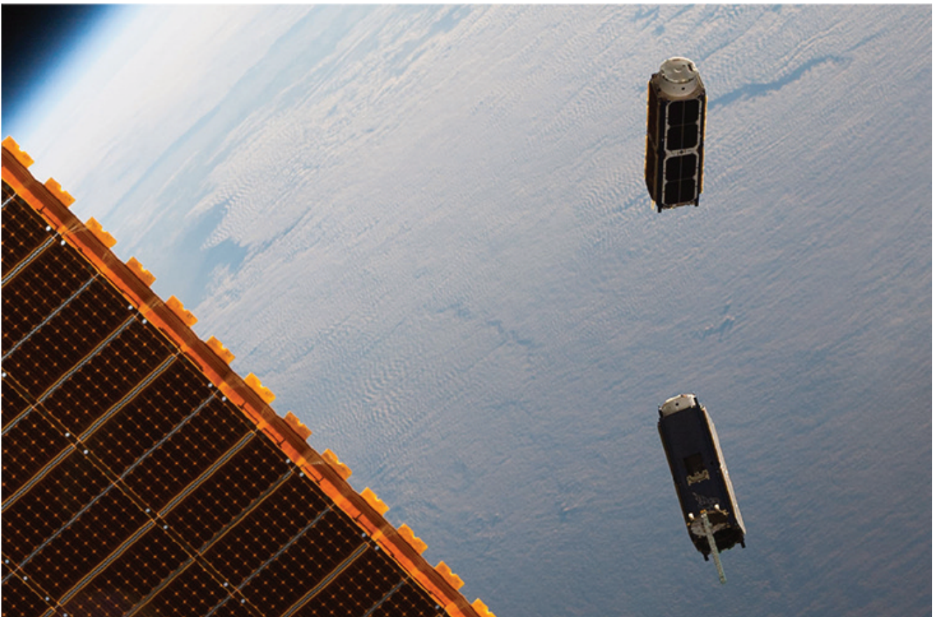
Figure 13.4.4 Two small CubeSat satellites deployed from the International Space Station in May, 2016. The solar sails open out when the CubeSats are far enough away from the Station.
