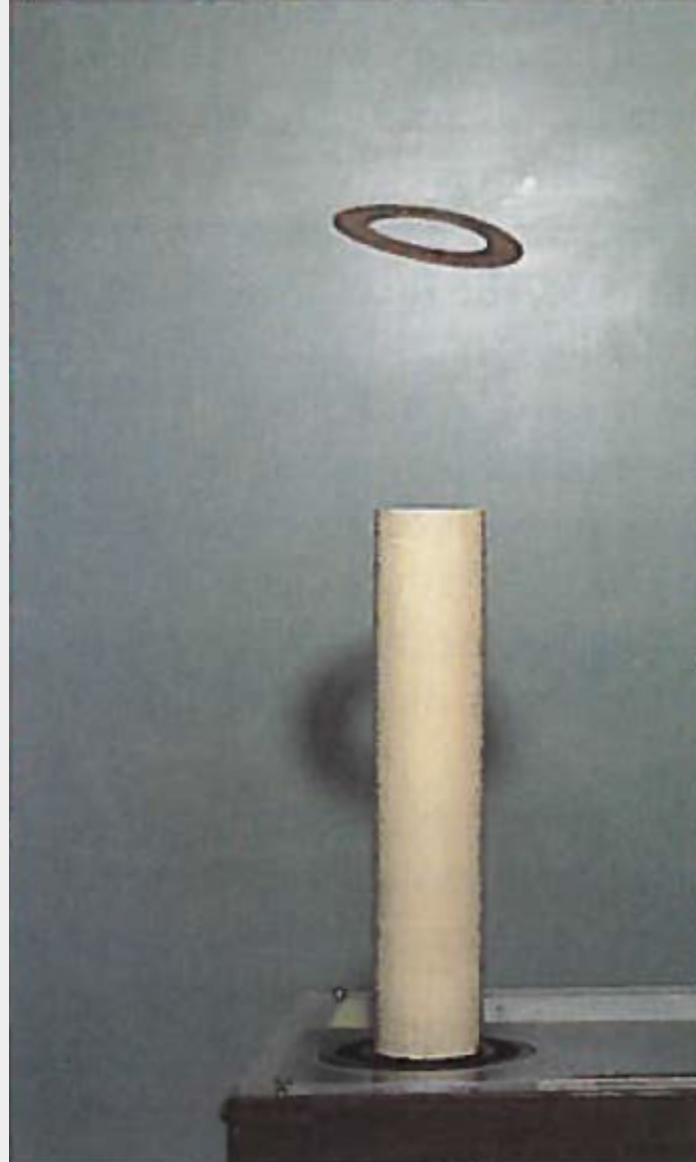
Figure 10.2.4 The jumping ring. When a current is turned on in the vertical solenoid, a current is induced in the metal ring. The stray field produced by the solenoid causes the ring to jump off the solenoid.
