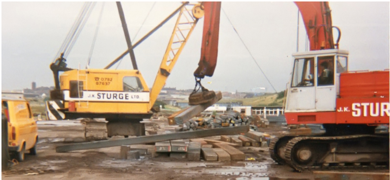
Figure 8.0.1. An industrial electromagnet is capable of lifting thousands of pounds of metallic waste. (credit: modification of work by “BedfordAI”/Flickr)
