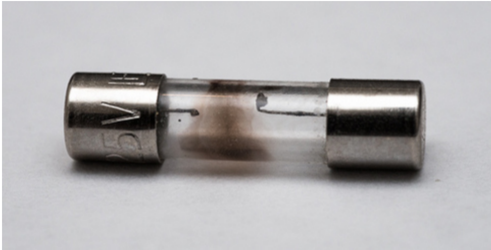
Figure 5.5.3 A fuse consists of a piece of wire between two contacts. When a current passes through the wire that is greater than the rated current, the wire melts, breaking the connection. Pictured is a “blown” fuse where the wire broke protecting a circuit (credit: modification of work by “Shardayy”/Flickr).
