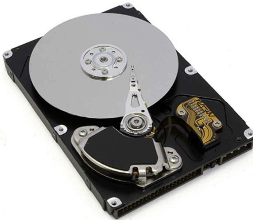
Figure 9.7.6 The inside of a hard disk drive. The silver disk contains the information, whereas the thin stylus on top of the disk reads and writes information to the disk.
