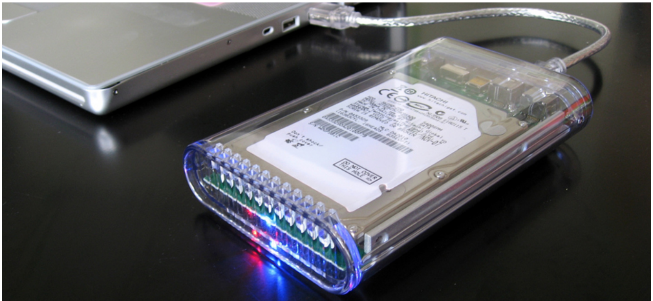
Figure 9.0.1. An external hard drive attached to a computer works by magnetically encoding information that can be stored or retrieved quickly. A key idea in the development of digital devices is the ability to produce and use magnetic fields in this way. (credit: modification of work by “Miss Karen”/Flickr)
