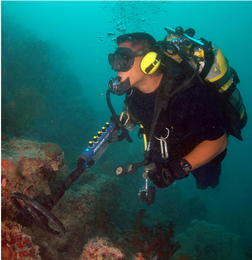
Figure 12.5.3 When a metal detector comes near a piece of metal, the self-inductance of one of its coils changes. This causes a shift in the resonant frequency of a circuit containing the coil. That shift is detected by the circuitry and transmitted to the diver by means of the headphones.
