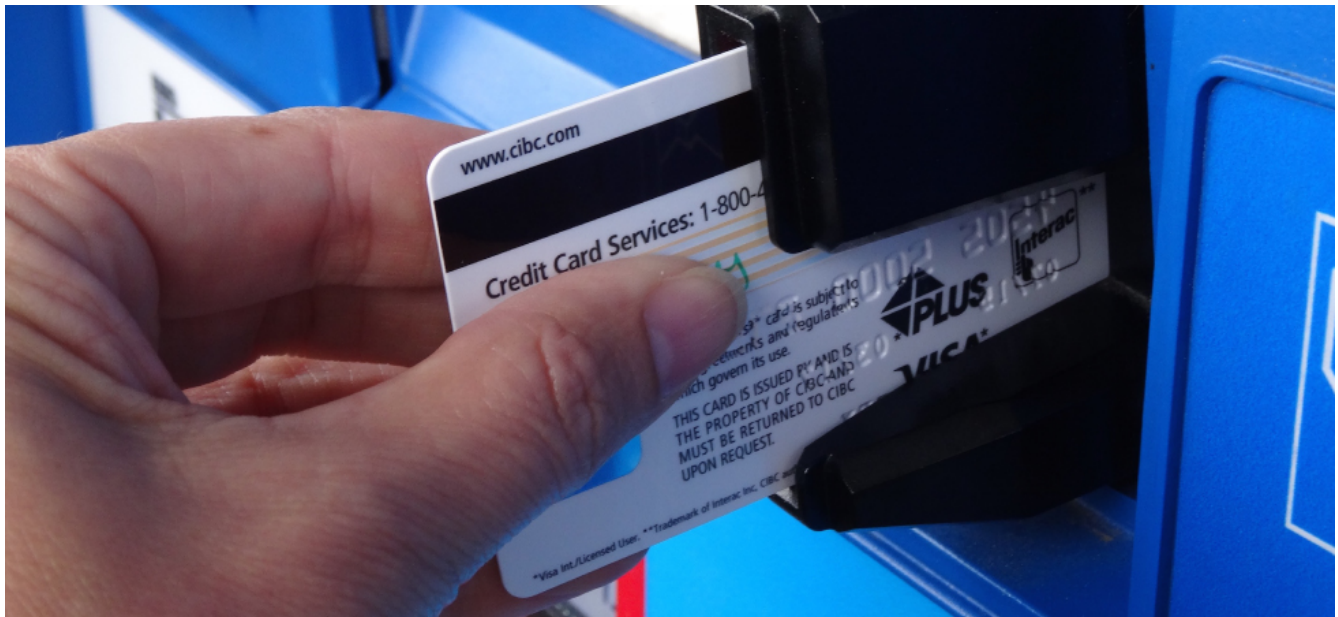
Figure 10.0.1. The black strip found on the back of credit cards and driver's licenses is a very thin layer of magnetic material with information stored on it. Reading and writing the information on the credit card is done with a swiping motion. The physical reason why this is necessary is called electromagnetic induction and is discussed in this chapter.
