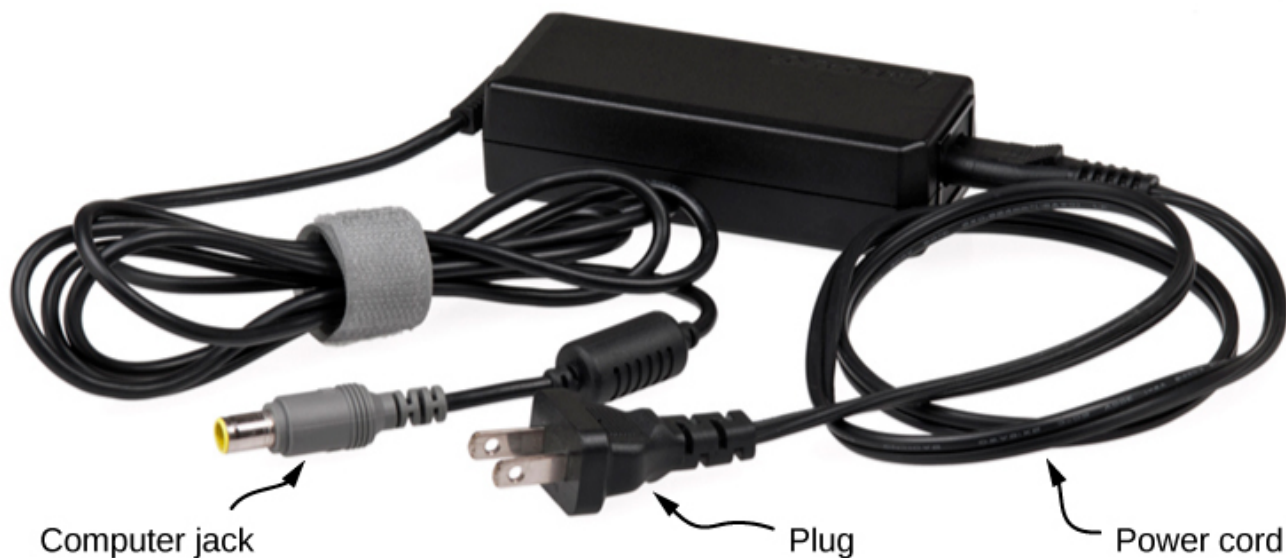
Figure 1.2.1. This power adapter uses metal wires and connectors to conduct electricity from the wall socket to a laptop computer. The conducting wires allow electrons to move freely through the cables, which are shielded by rubber and plastic. These materials act as insulators that don't allow electric charge to escape outward. (credit: modification of work by "Evan-Amos"/Wikimedia Commons)
