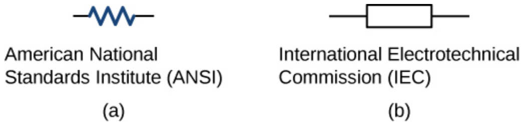
Figure 5.3.2 Symbols for a resistor used in circuit diagrams. (a) The ANSI symbol; (b) the IEC symbol.
