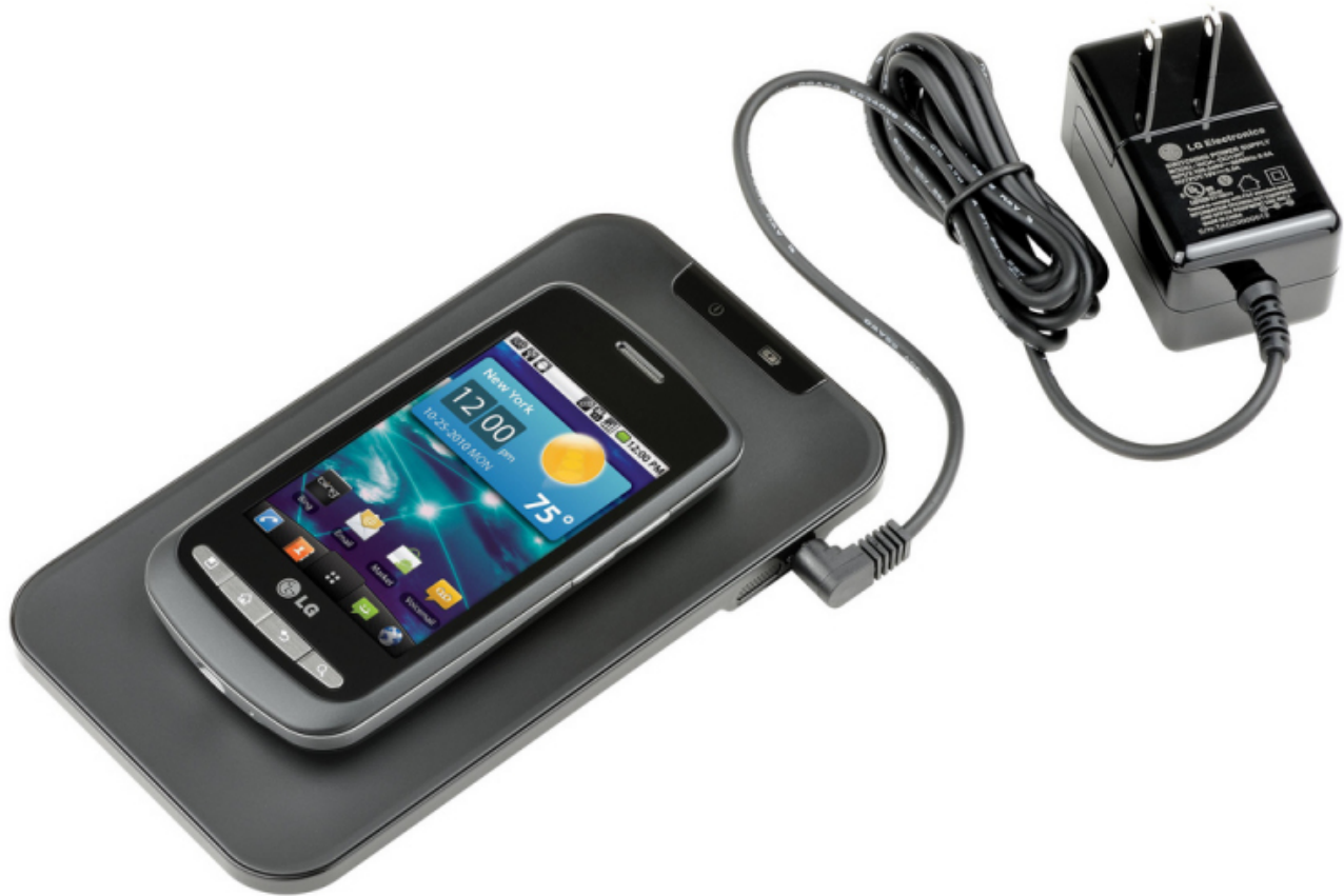
Figure 11.0.1. A smartphone charging mat contains a coil that receives alternating current, or current that is constantly increasing and decreasing. The varying current induces an emf in the smartphone, which charges its battery. Note that the black box containing the electrical plug also contains a transformer (discussed in Alternating-Current Circuits) that modifies the current from the outlet to suit the needs of the smartphone. (credit: modification of work by “LG”/Flickr)
