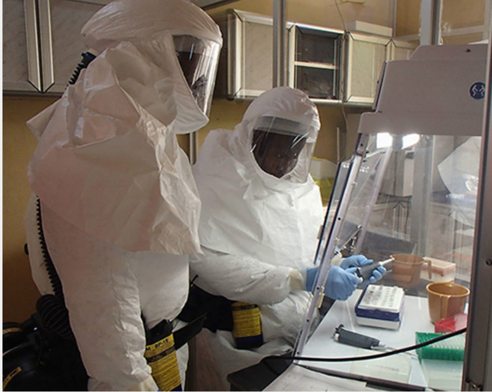
Figure 6.15. Researchers working with Ebola virus use layers of defences against accidental infection, including protective clothing, breathing systems, and negative air-pressure cabinets for bench work. (credit: modification of work by Randal J. Schoepp)
