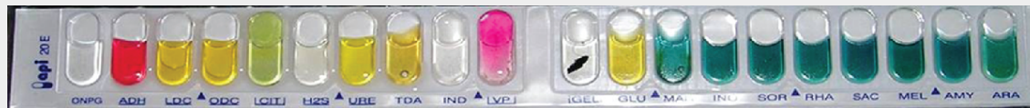
Figure 8.24. The API 20NE test strip is used to identify specific strains of gram-negative bacteria outside the Enterobacteriaceae. Here is an API 20NE test strip result for Photobacterium damsela ssp. piscicida .
