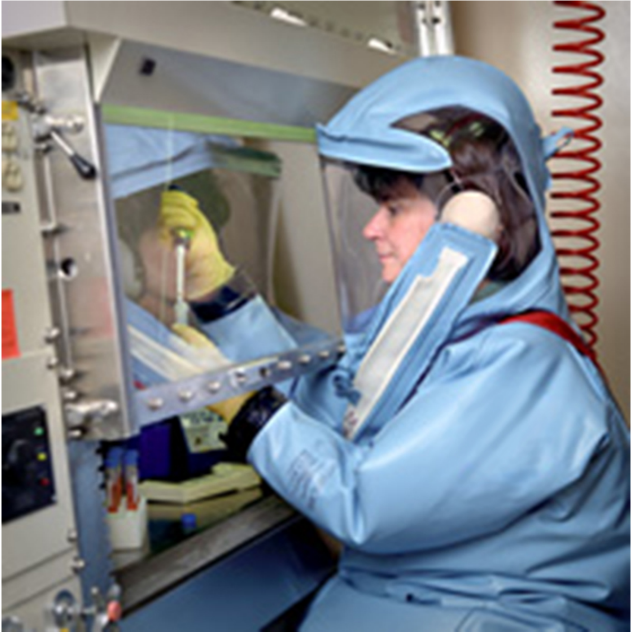
Figure 14.2. A protective suit like this one is an additional precaution for those who work in BSL-4 laboratories. This suit has its own air supply and maintains a positive pressure relative to the outside, so that if a leak occurs, air will flow out of the suit, not into it from the laboratory. (credit: modification of work by Centers for Disease Control and Prevention)
